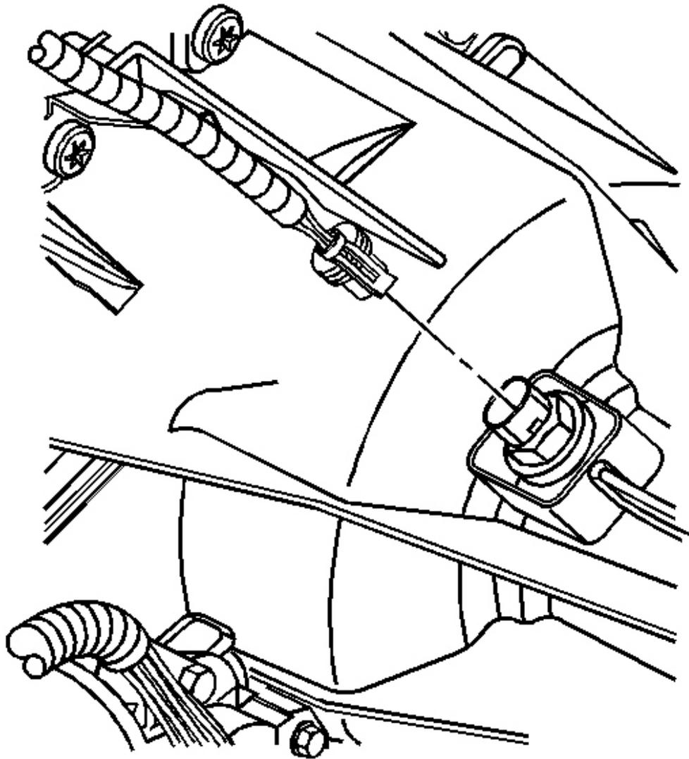
**Fig. 18: Electrical Connector & Speed Sensor**
