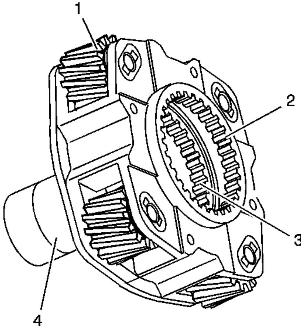
**Fig. 58: View Of High/Low Planetary Carrier Inspection Areas**
