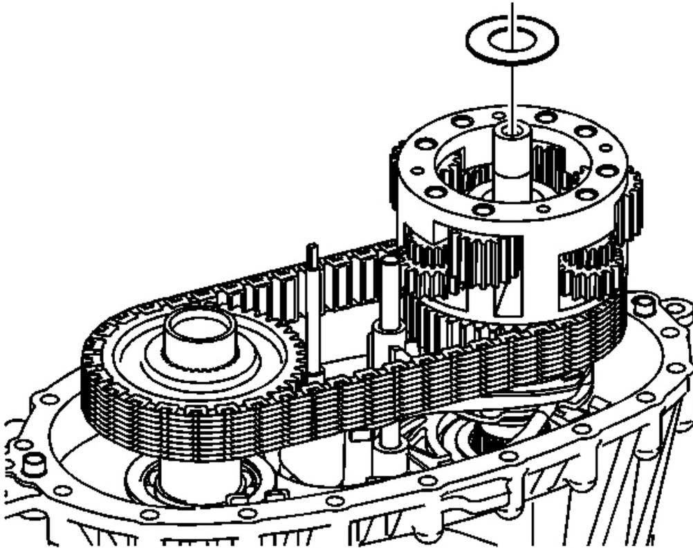
**Fig. 17: Locating Rear Output Shaft Thrust Washer**
