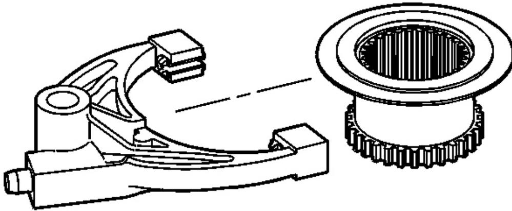
**Fig. 69: Range Shift Fork Range Shift Sleeve**
