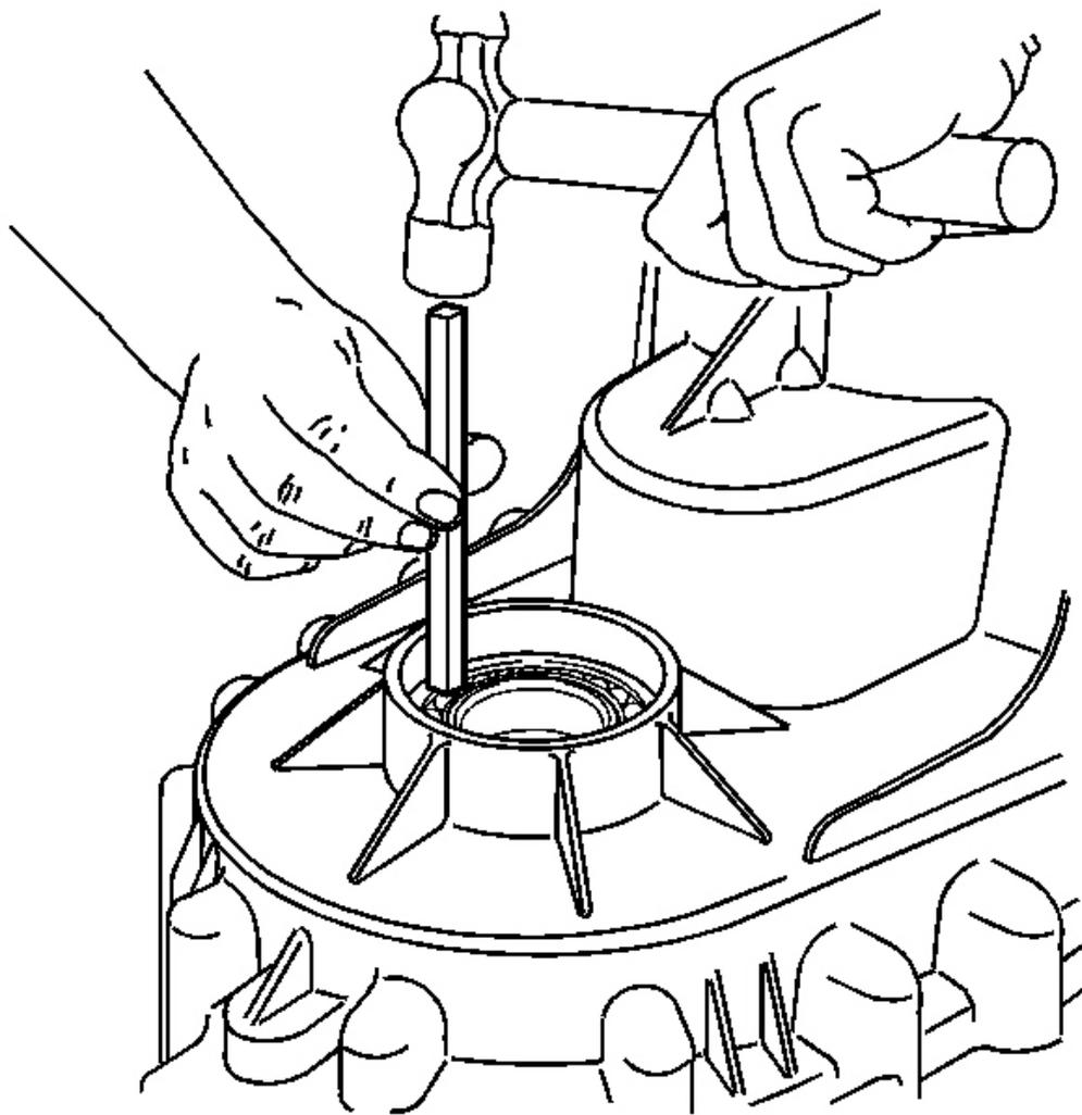
**Fig. 77: Removing Front Output Shaft Bearing From Front Case Half By Using Brass Drift**
