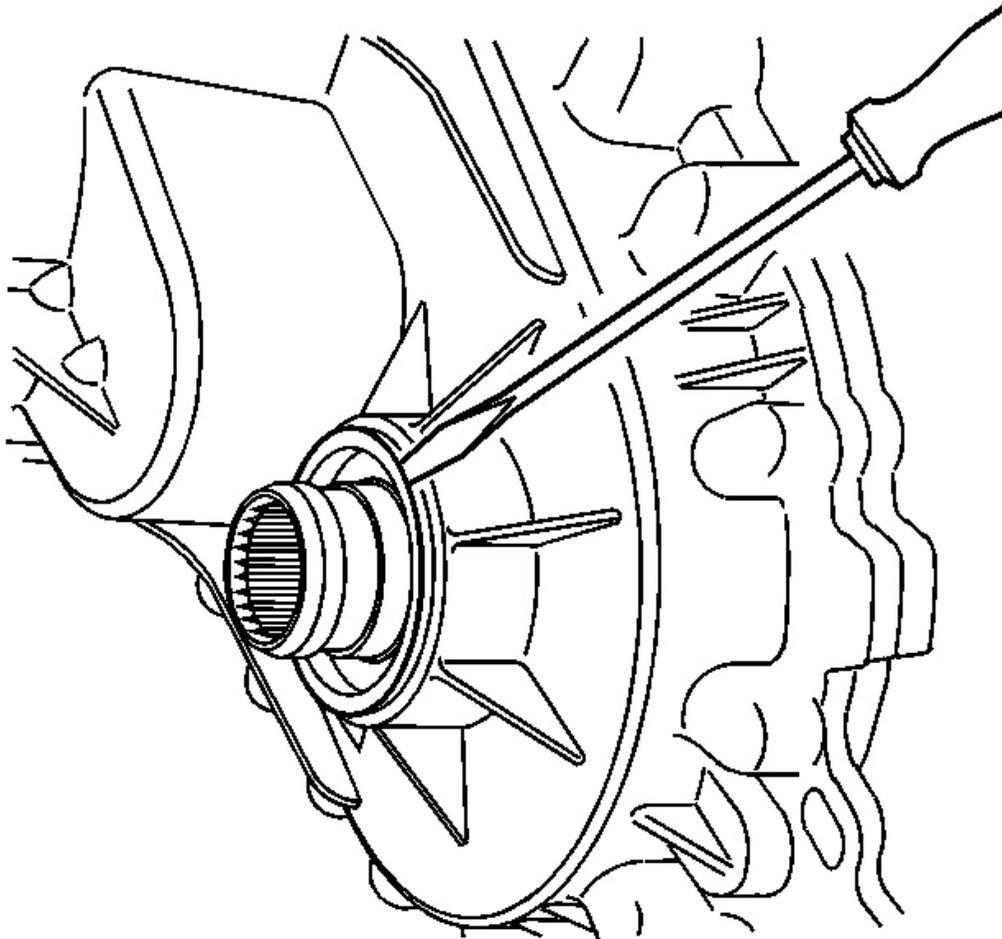
**Fig. 19: Prying Inner Seal Race Forward**
