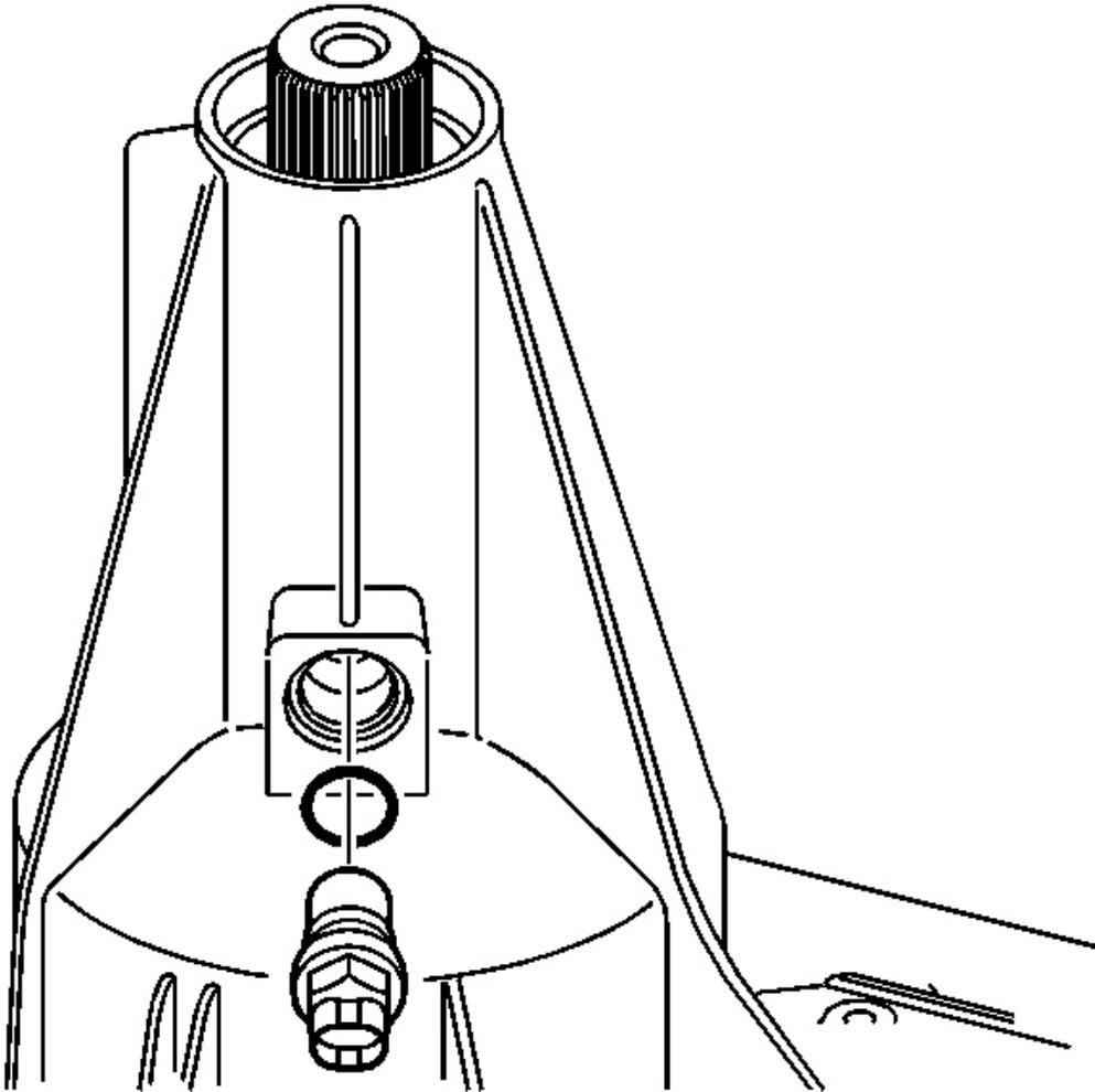
**Fig. 149: Installing Vehicle Speed Sensor With New O-Ring Seal**
