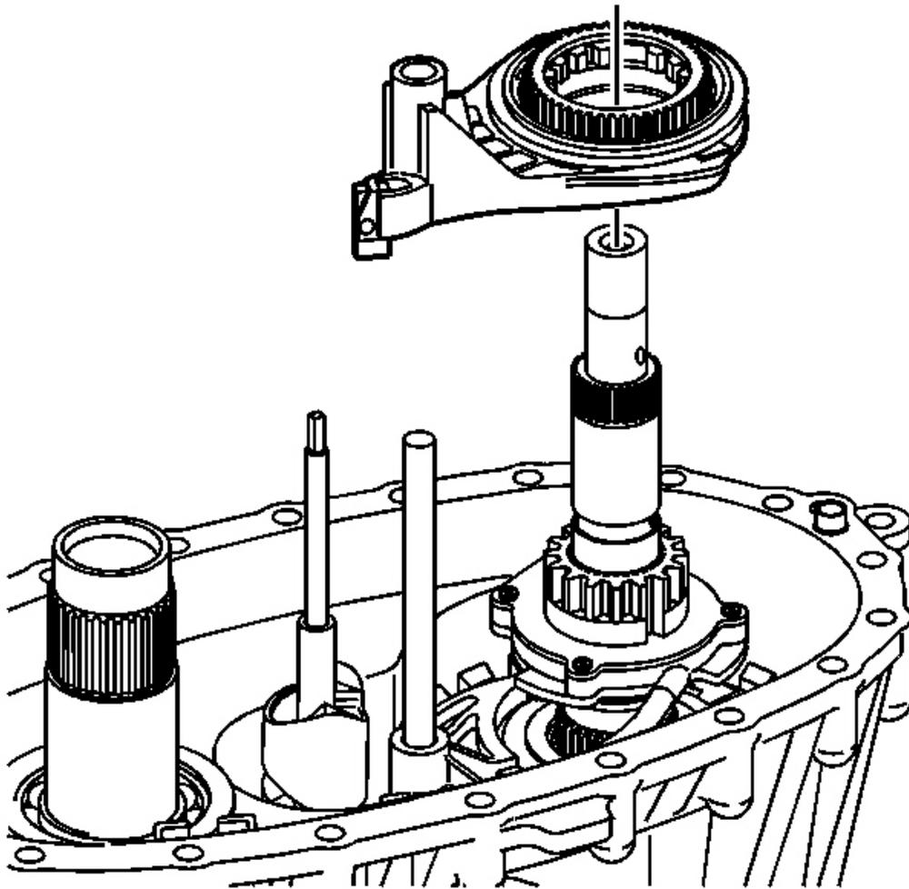
**Fig. 95: Identifying Lockup Shift Assembly & Lockup Mode Shift Fork**
