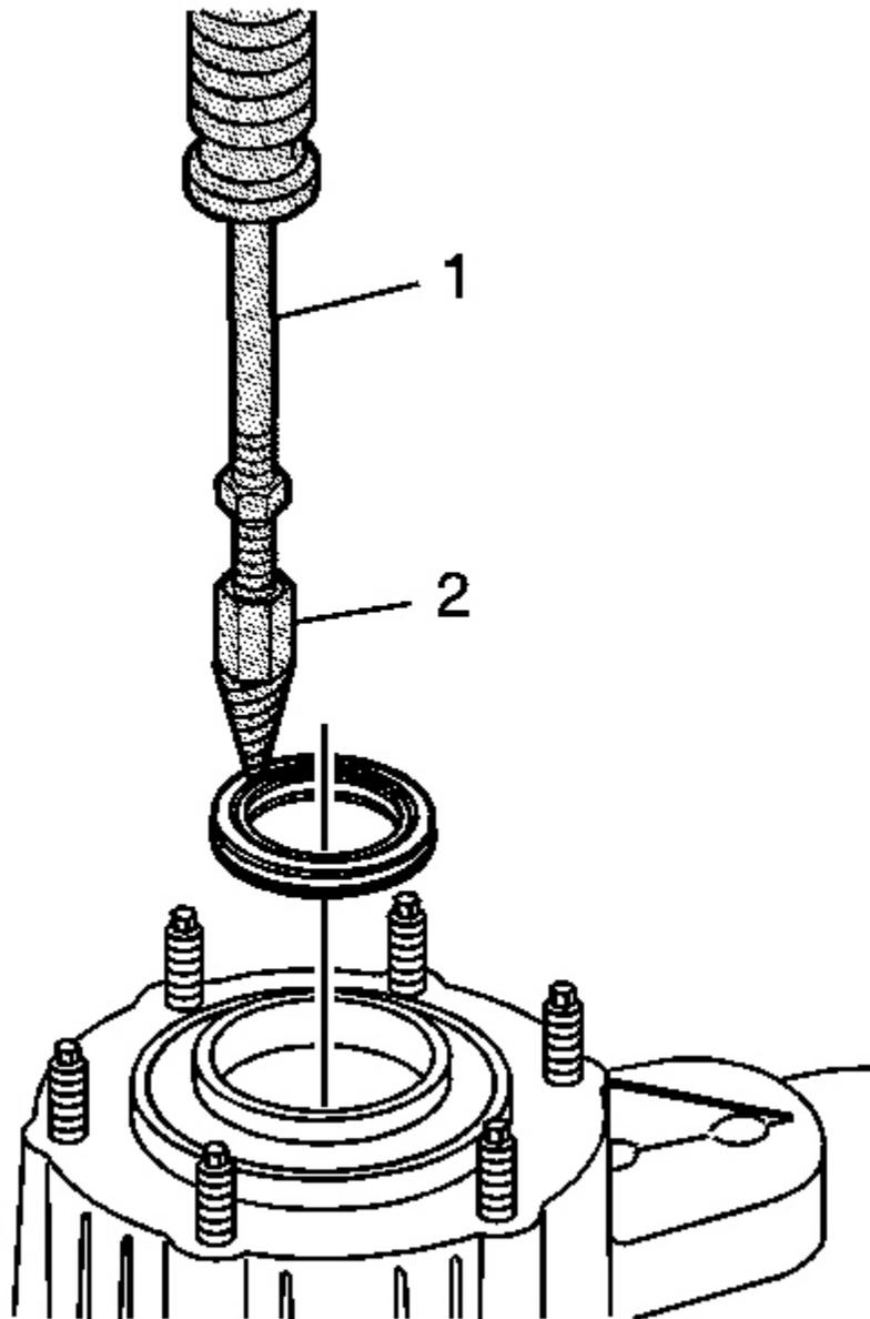
**Fig. 30: Using J 36825 To Remove Input Shaft Seal From Transfer Case**
