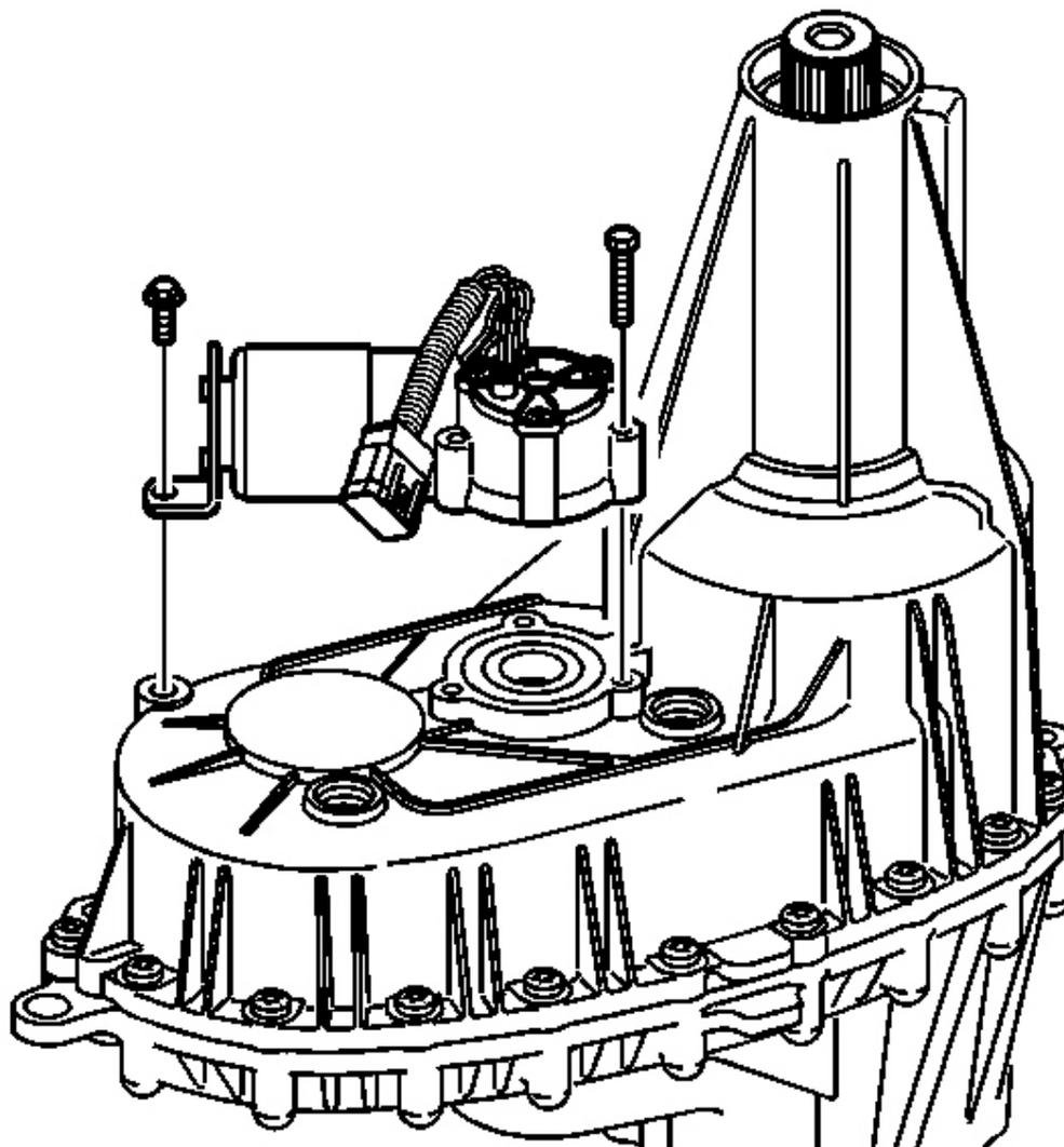
**Fig. 115: Identifying Encoder Motor Assembly**
