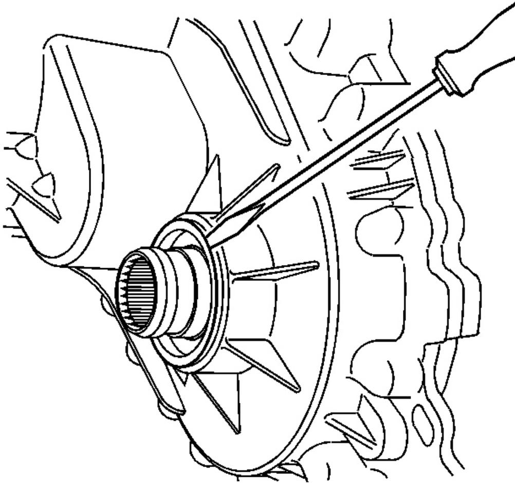
**Fig. 6: Inserting Screwdriver Behind Inner Race Of Seal**
