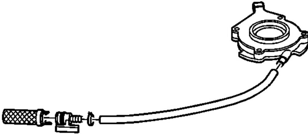
**Fig. 89: Locating Oil Pump Hose & Screen**
