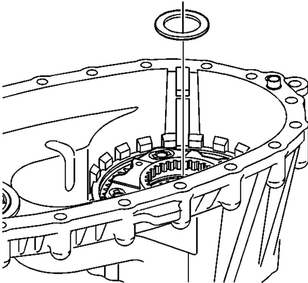
**Fig. 35: Locating Input Shaft Thrust Washer**
