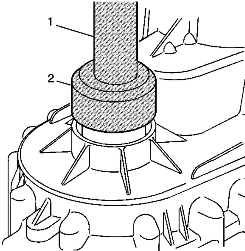
**Fig. 22: Using J 43484 & J 8092 To Install Transfer Case Output Seal**
