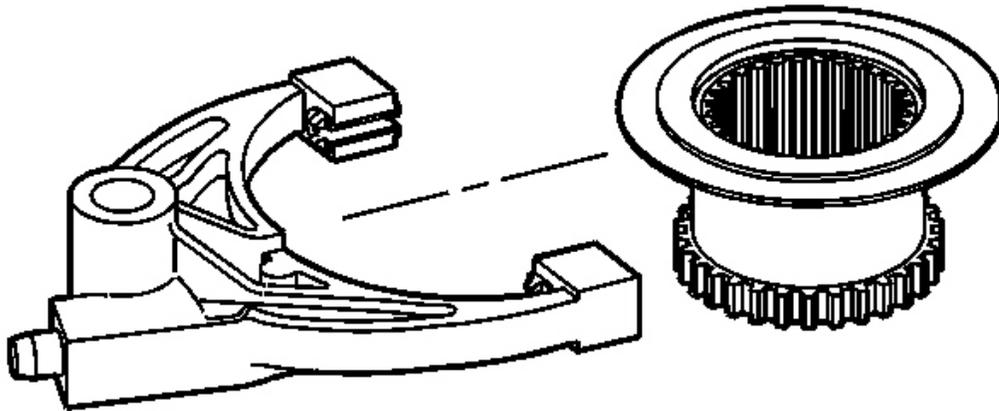
**Fig. 34: View Of Range Shift Fork & Range Shift Sleeve**
