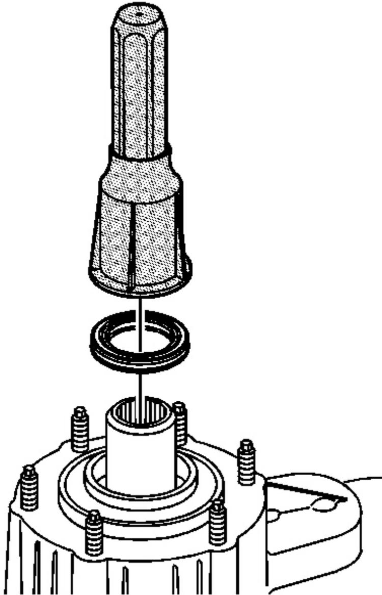
**Fig. 31: Using J 42738 To Install Input Shaft Seal In Transfer Case**
