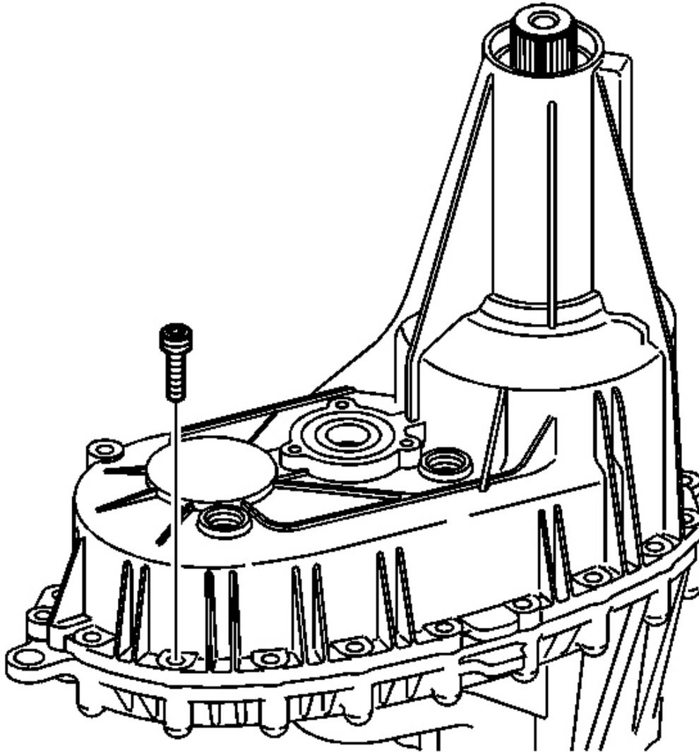
**Fig. 113: Identifying Transfer Case Retaining Bolts**
