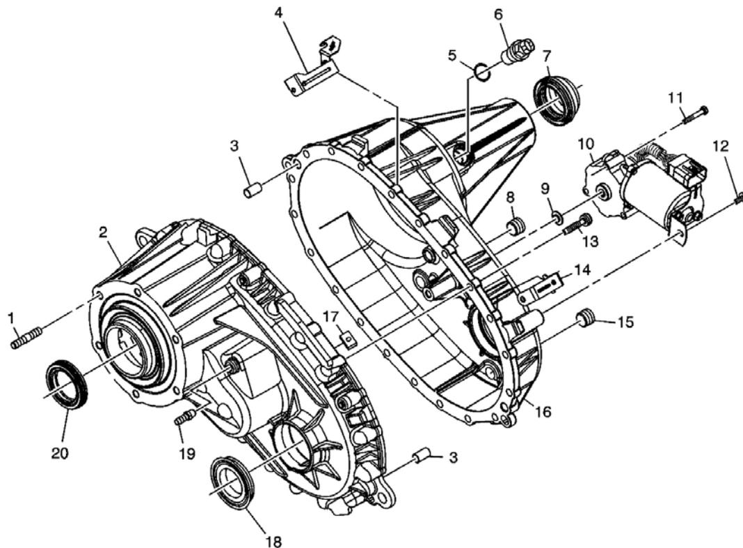
**Fig. 1: Transfer Case Component Views**
