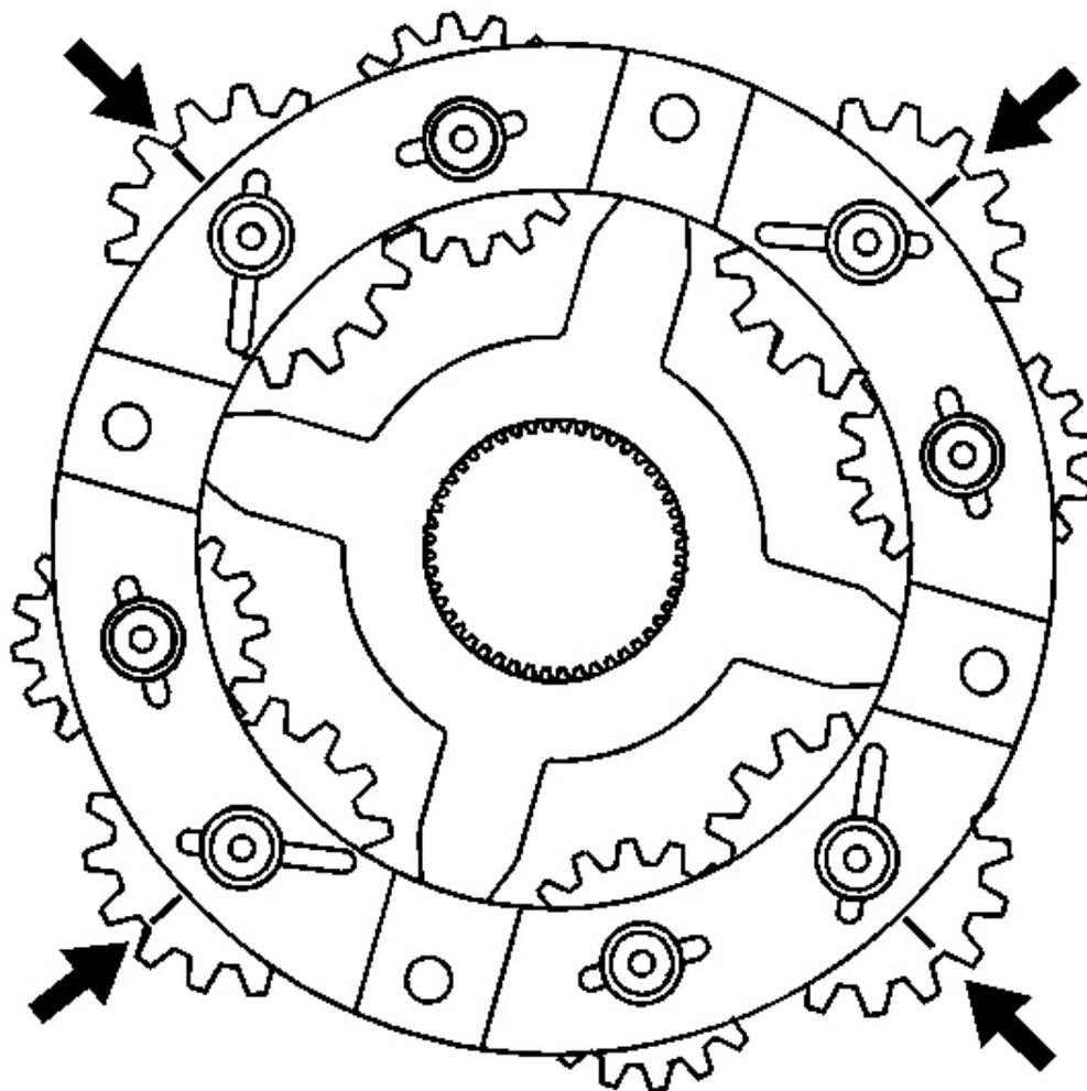
**Fig. 134: Aligning Marks On Pinion Gears**
