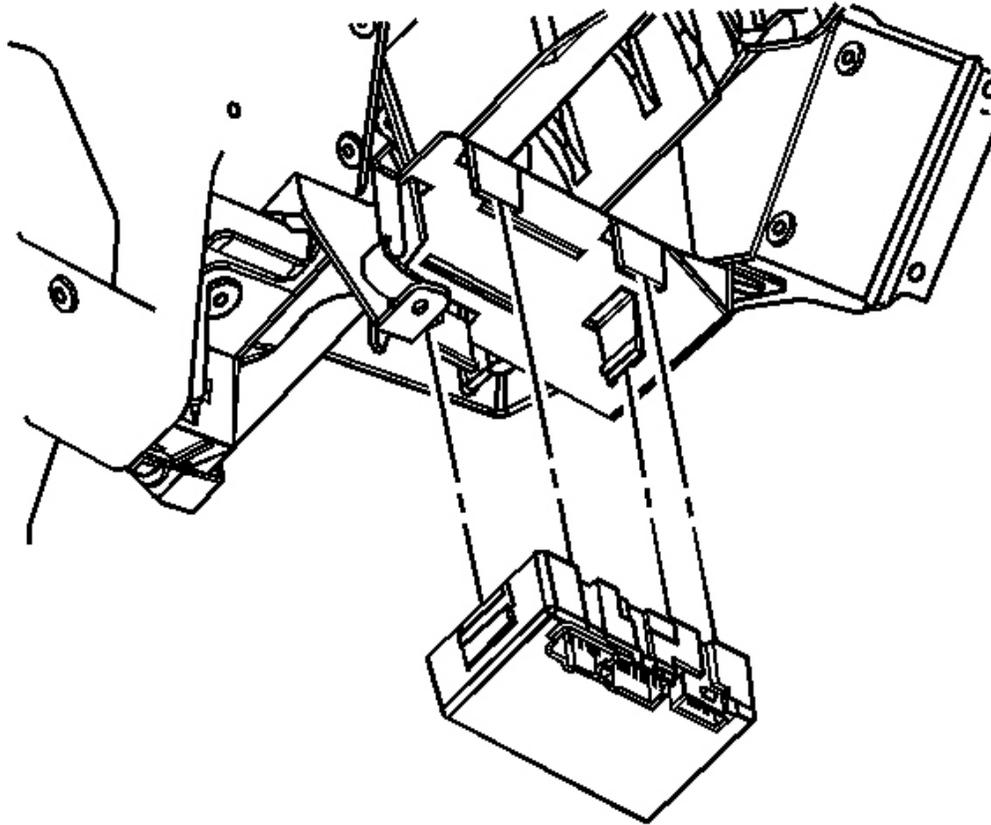
**Fig. 160: Transfer Case Shift Control Module**
