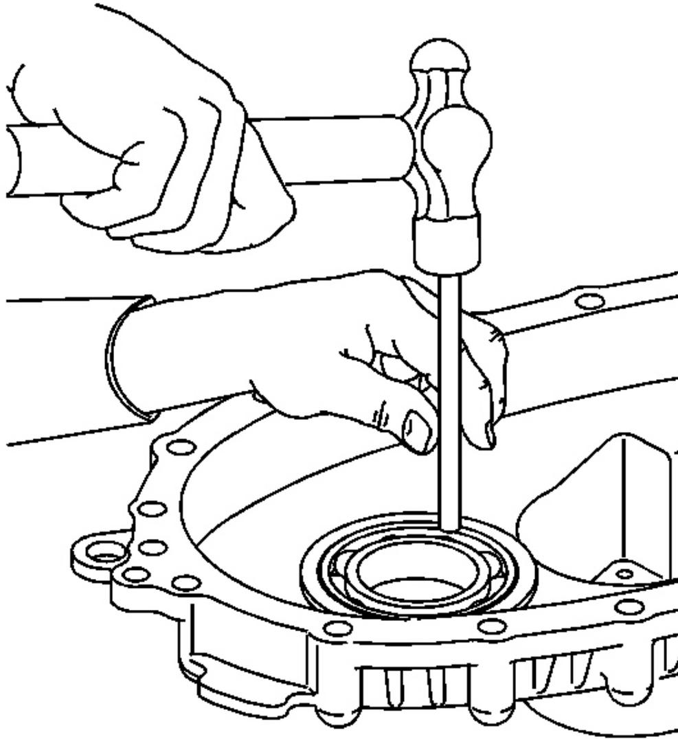
**Fig. 112: Installing Front Bearing**
