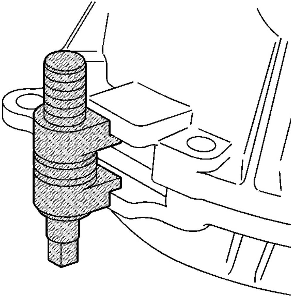
**Fig. 13: View Of J 45358 Installed Between The Tabs On The Case Halves**
