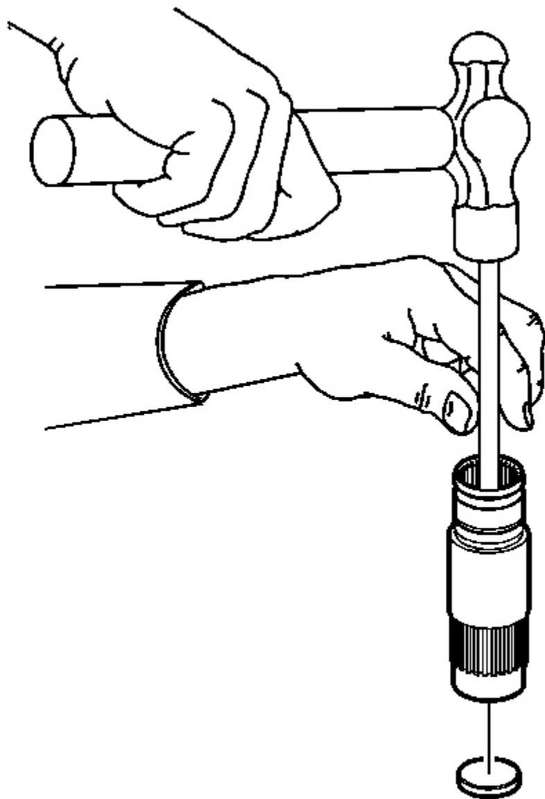
**Fig. 74: Removing Cup Plug In Front Output Shaft (If Leaking)**
