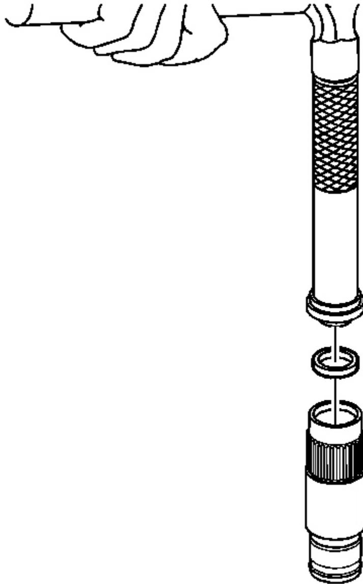
**Fig. 78: Installing Cup Plug**
