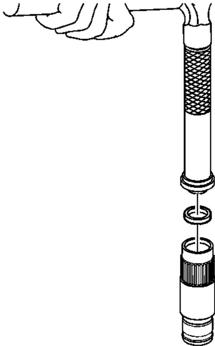
**Fig. 113: Installing Cup Plug In Front Output Shaft**
