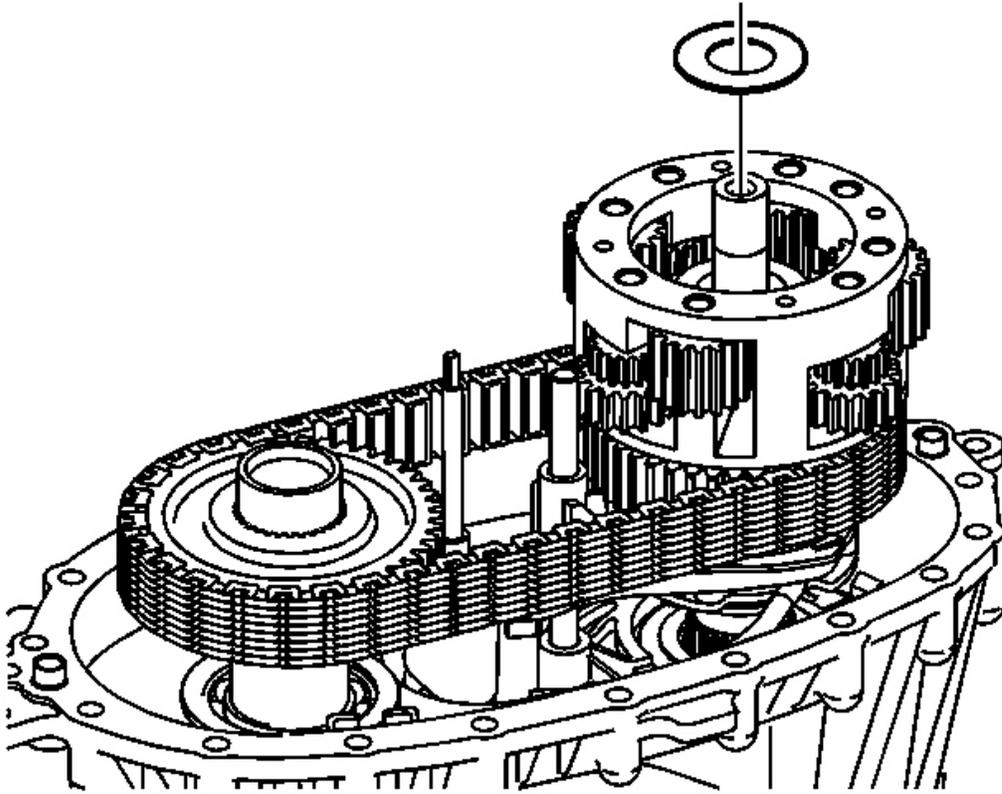
**Fig. 52: Rear Output Shaft Thrust Washer**
