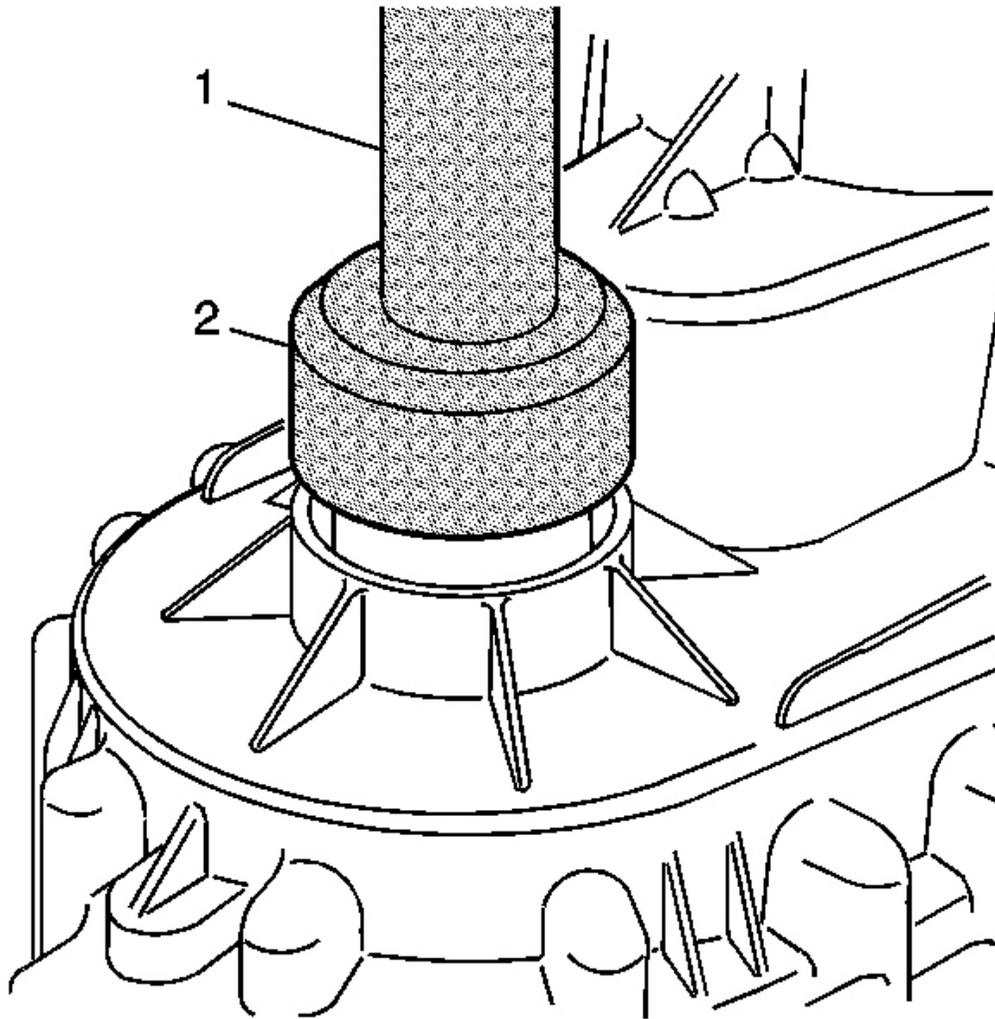
**Fig. 153: Using J 43484 & J 8092 To Install Transfer Case Output Seal**
