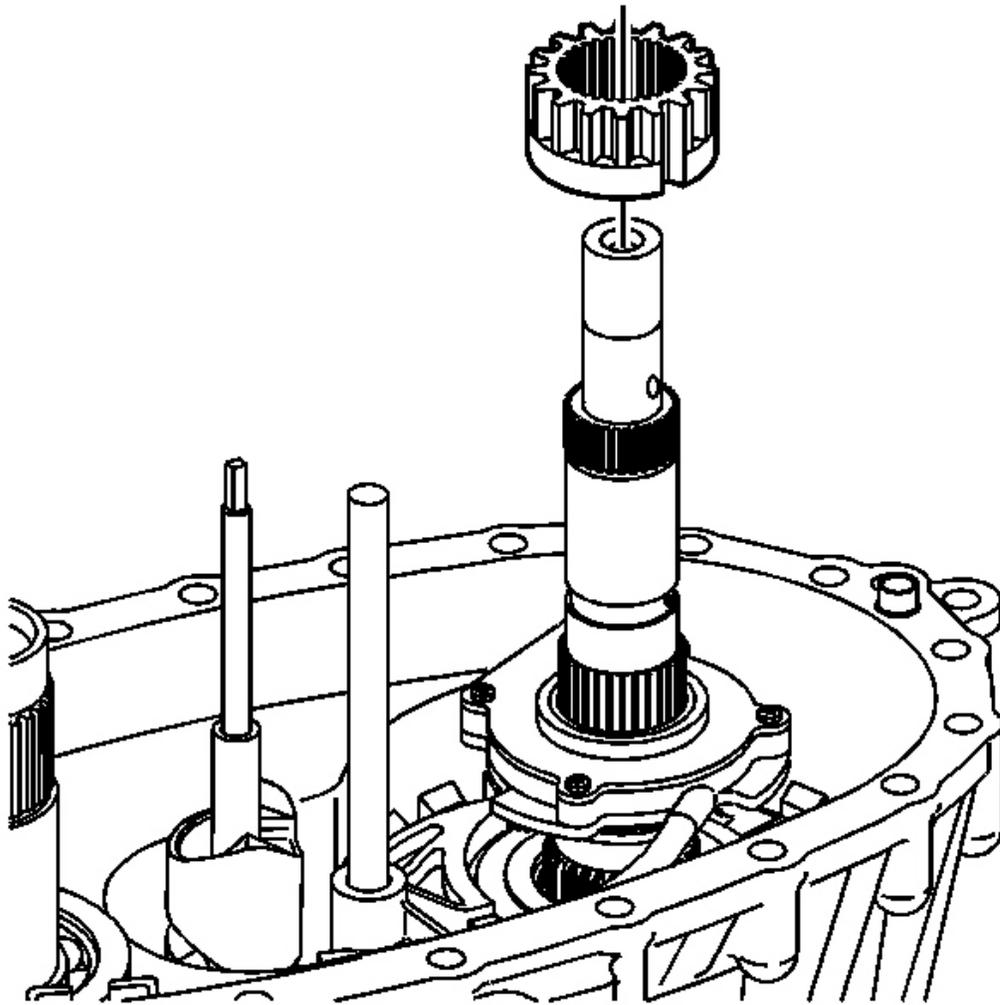
**Fig. 25: View Of Inner Lockup Hub**
