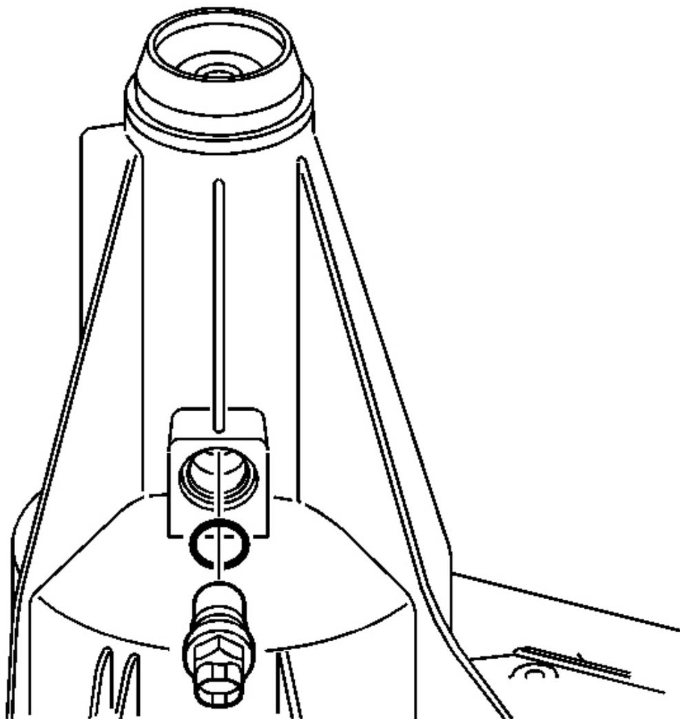
**Fig. 10: Identifying Vehicle Speed Sensor (VSS) & O-Ring Seal**
