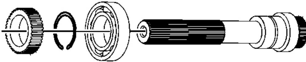
**Fig. 65: View Of Rear Output Shaft Components**
