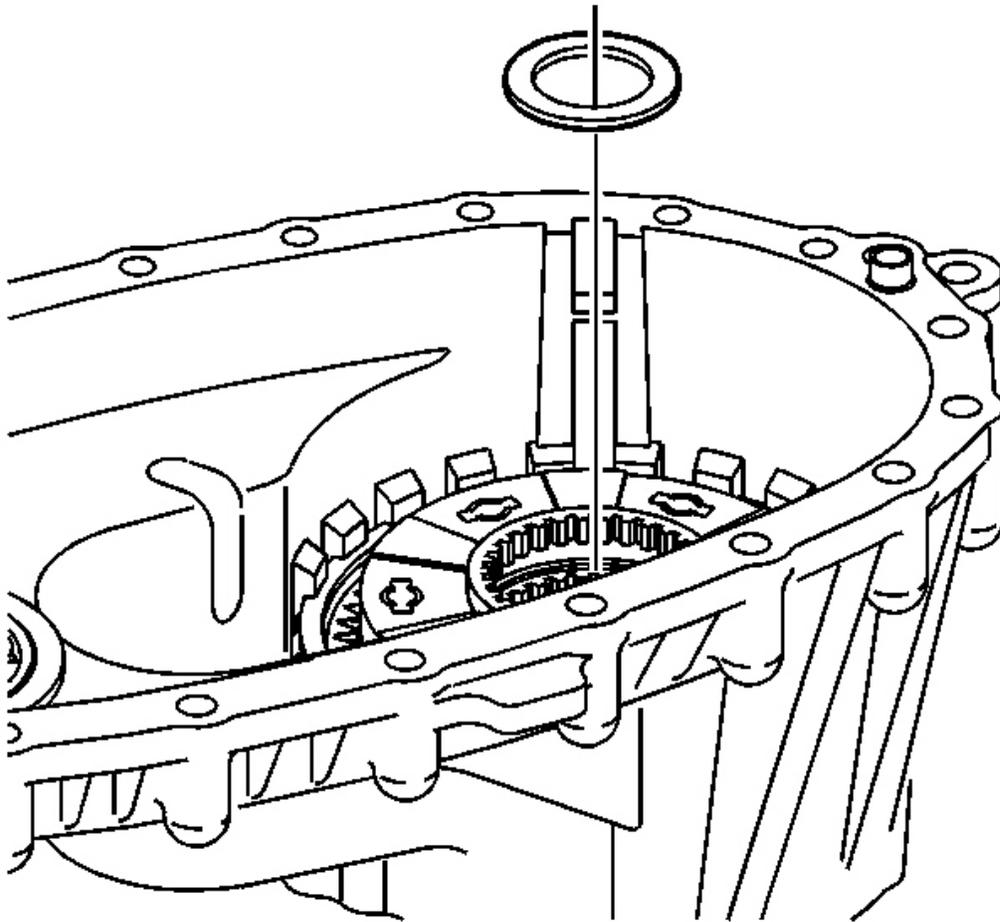
**Fig. 117: Input Shaft Thrust Washer**
