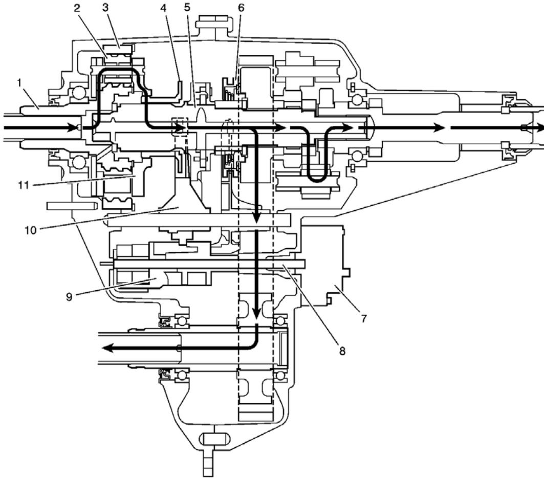
**Fig. 158: 4LO Lock Mode Power Flow**
