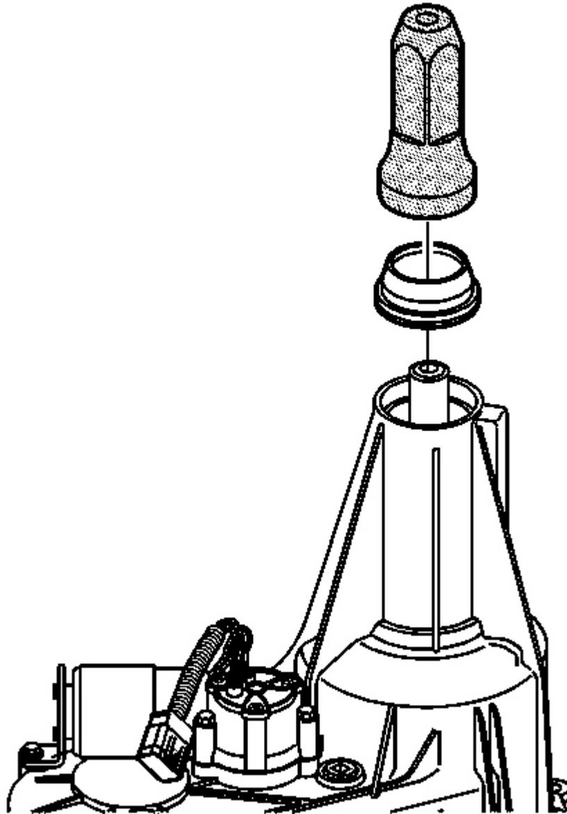
**Fig. 151: Installing Rear Output Shaft Seal By Using J 45756**
