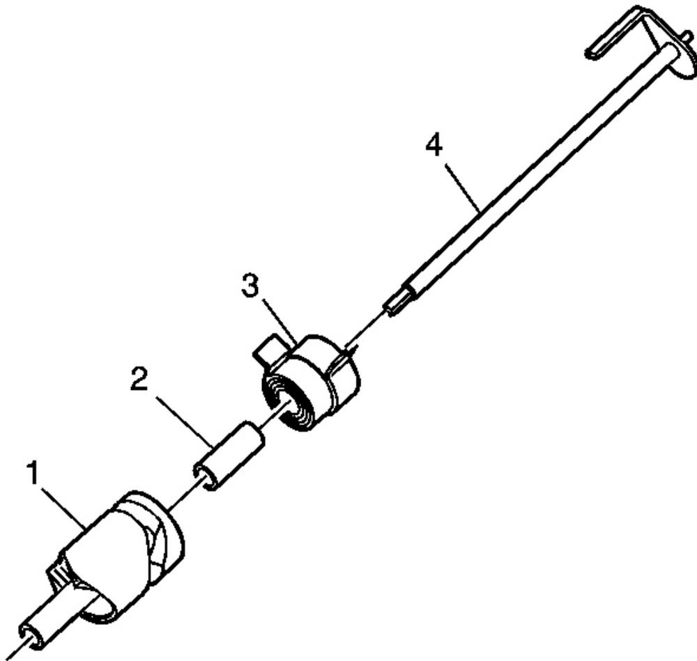
**Fig. 121: Shift Detent Lever Assembly Components**
