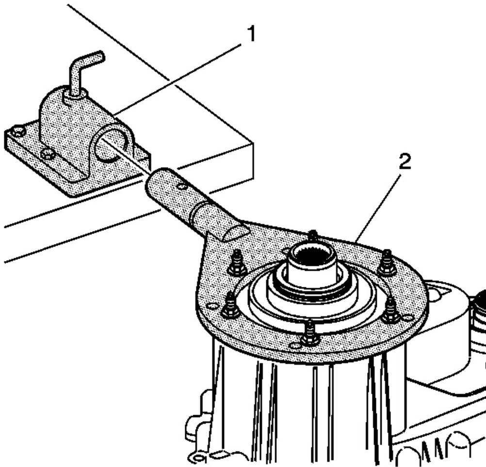
**Fig. 4: Installing J 45759 Into J 3289-20**
