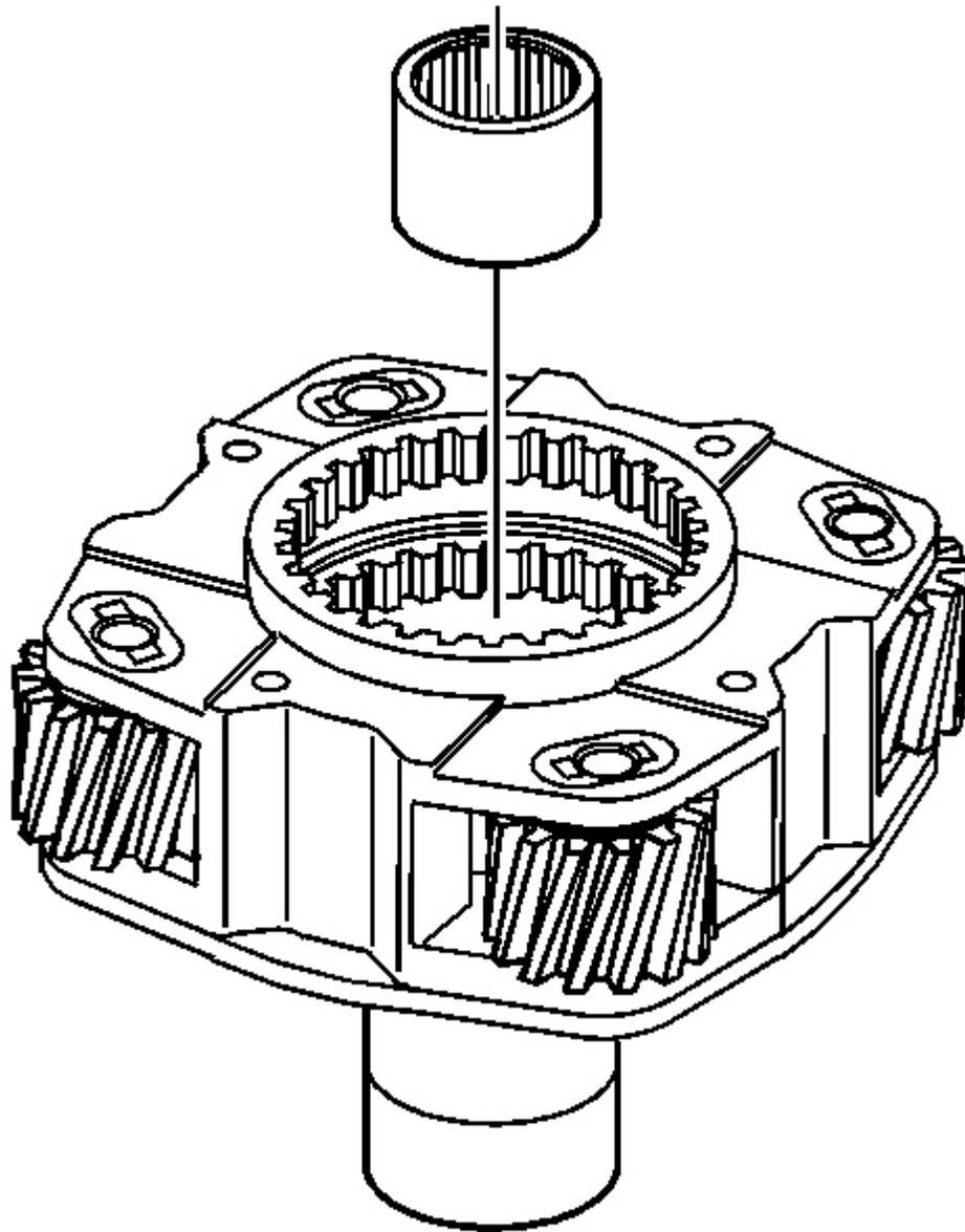
**Fig. 37: View Of Mainshaft Front Support Bearing**
