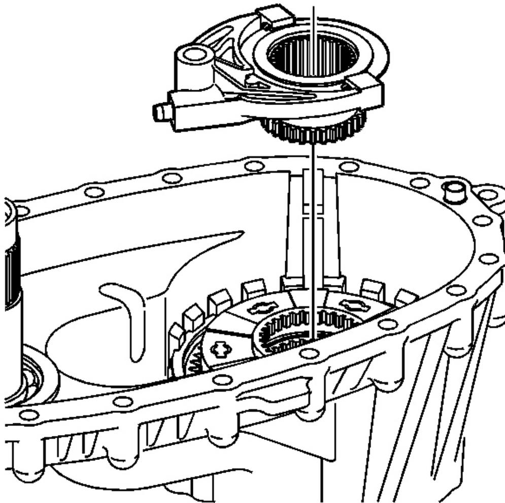
**Fig. 119: High/Low Range Sleeve & High/Low Range Shift Fork**
