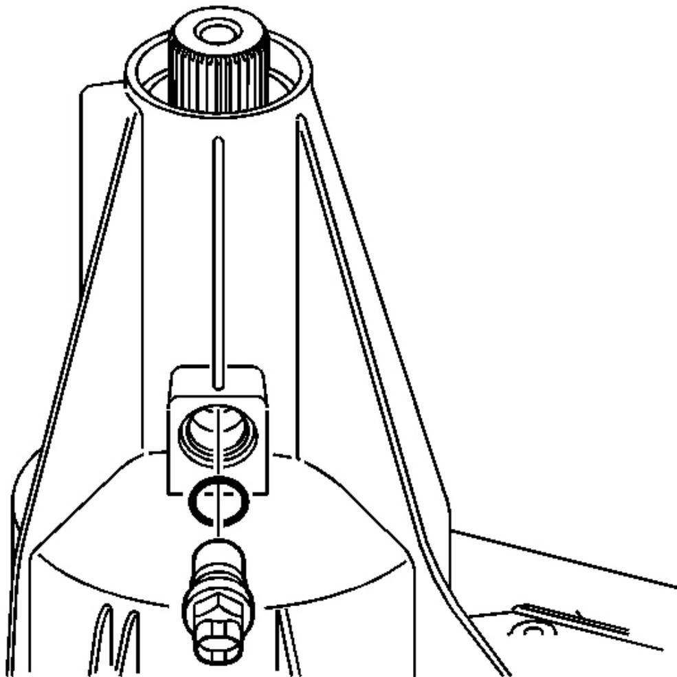
**Fig. 114: Locating Vehicle Speed Sensor (VSS)**
