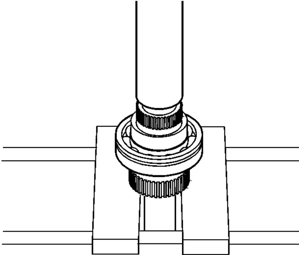
**Fig. 143: Installing NEW Speed Reluctor Wheel Using Hydraulic Press**
