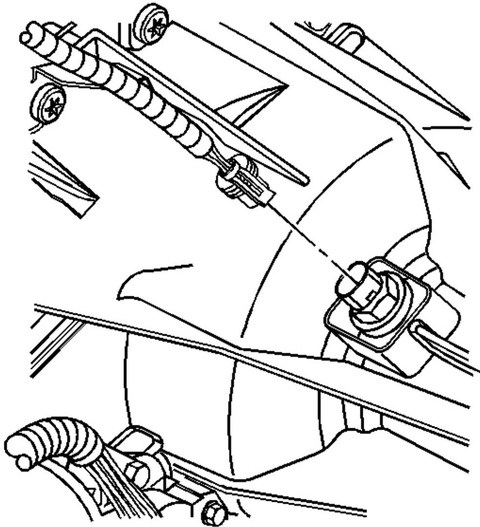
**Fig. 26: Electrical Connector & Speed Sensor**
