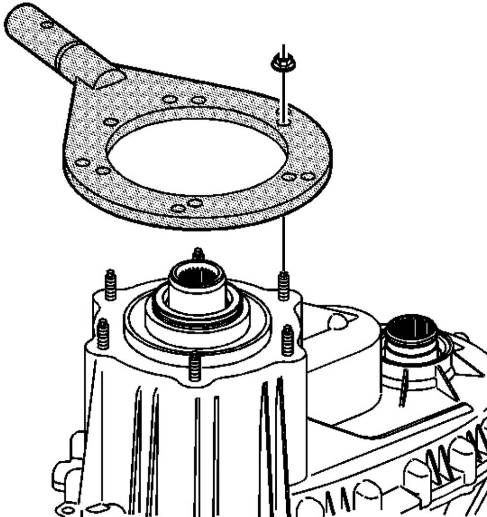
**Fig. 38: Attaching J 45759 To Transfer Case**
