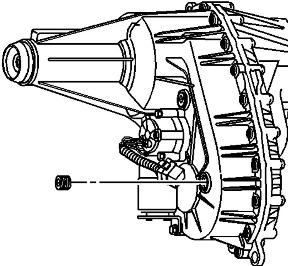
**Fig. 11: Transfer Case Drain Plug**
