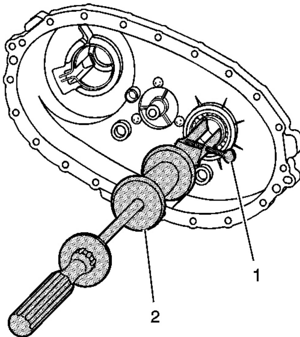
**Fig. 86: Using J 26941 & J 23907 To Remove Rear Bearing For Front Output Shaft From Rear Case**
