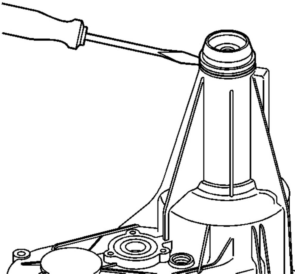
**Fig. 23: Rear Output Shaft Seal**
