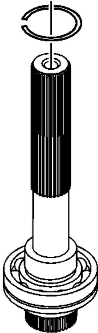
**Fig. 83: Retaining Ring & Rear Output Shaft Bearing**
