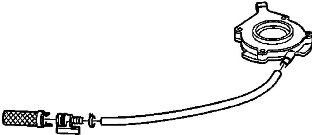
**Fig. 124: Oil Pump Hose & Oil Pump Screen**
