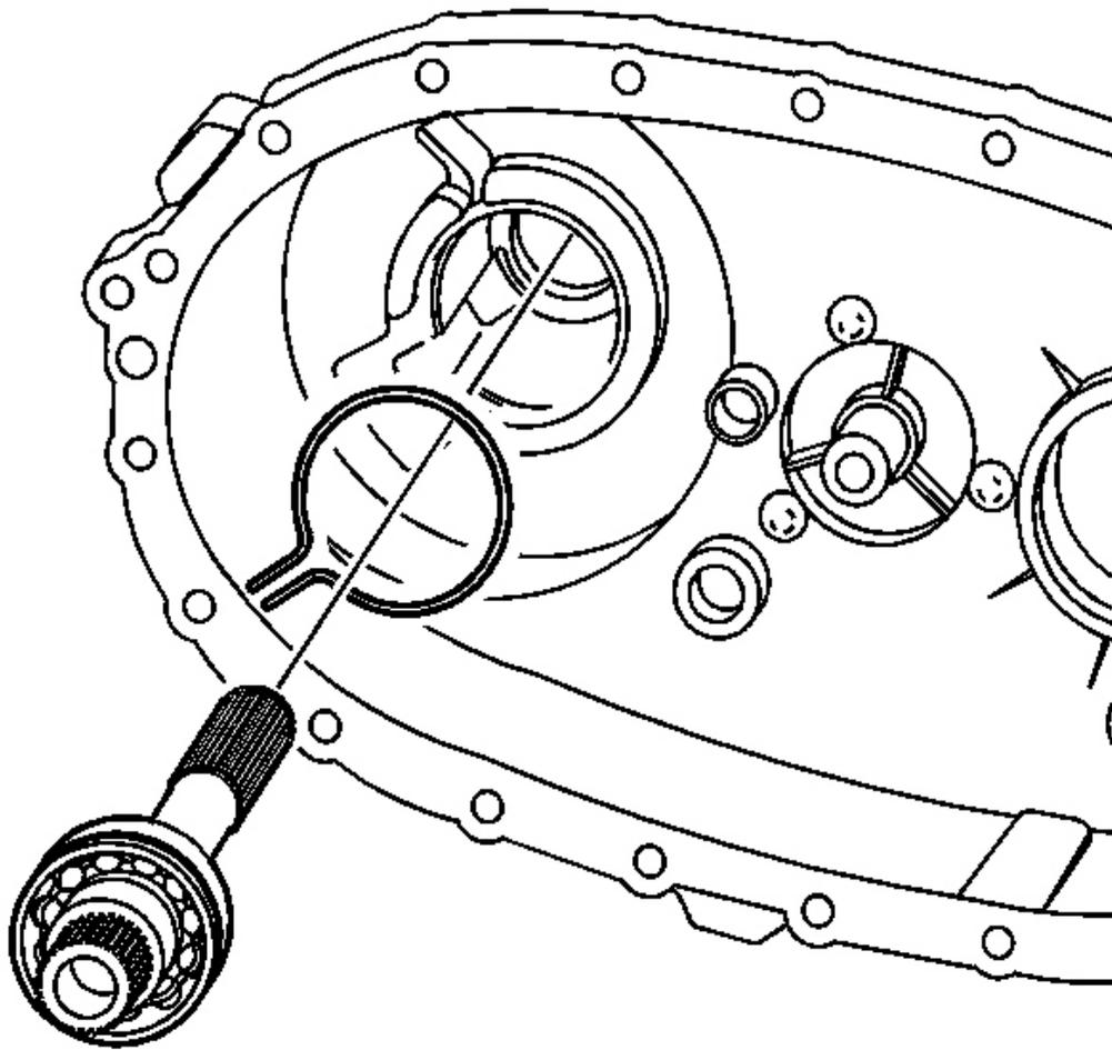
**Fig. 145: Rear Output Shaft & Rear Case Half**
