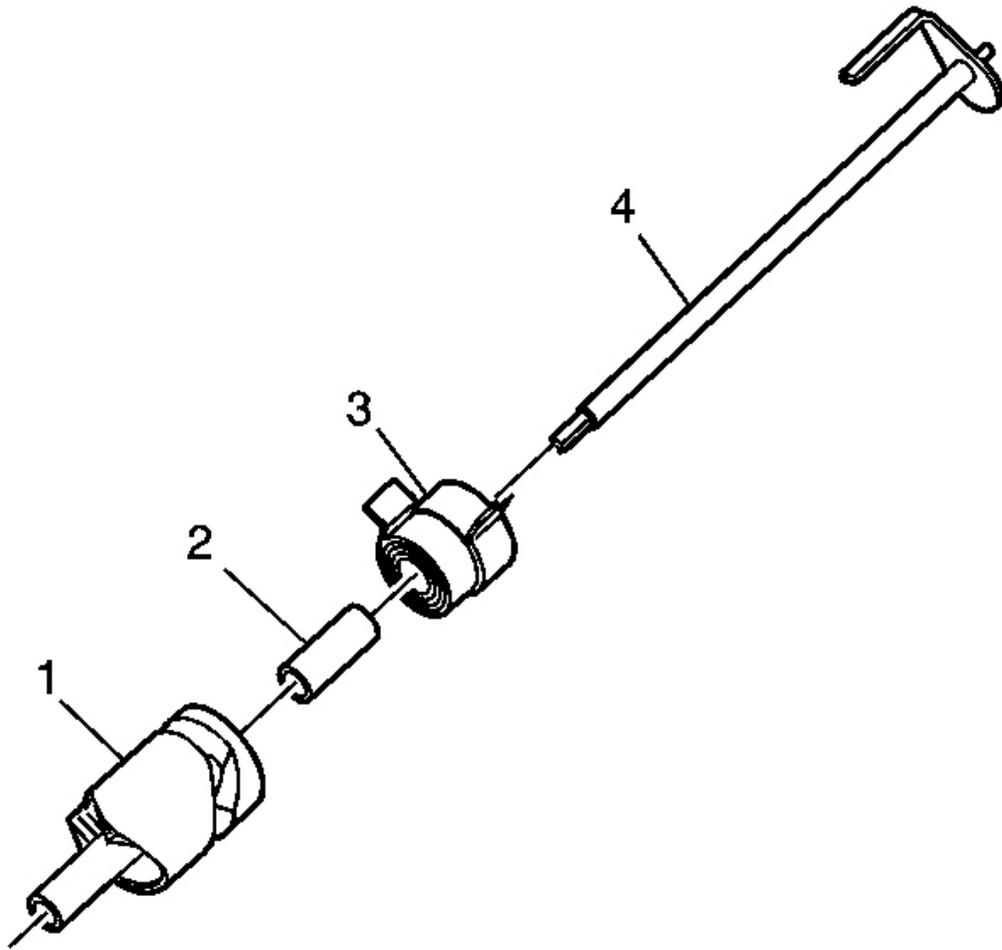
**Fig. 86: Expanded View Of Shift Detent Lever Assembly**
