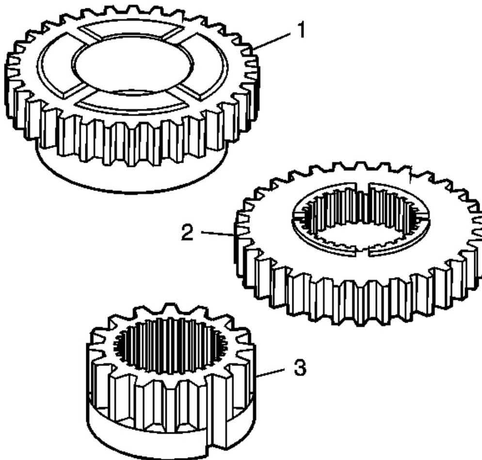
**Fig. 95: Inspecting Teeth On Front Sun Gear, Rear Sun Gear & Inner Lockup Hub**
