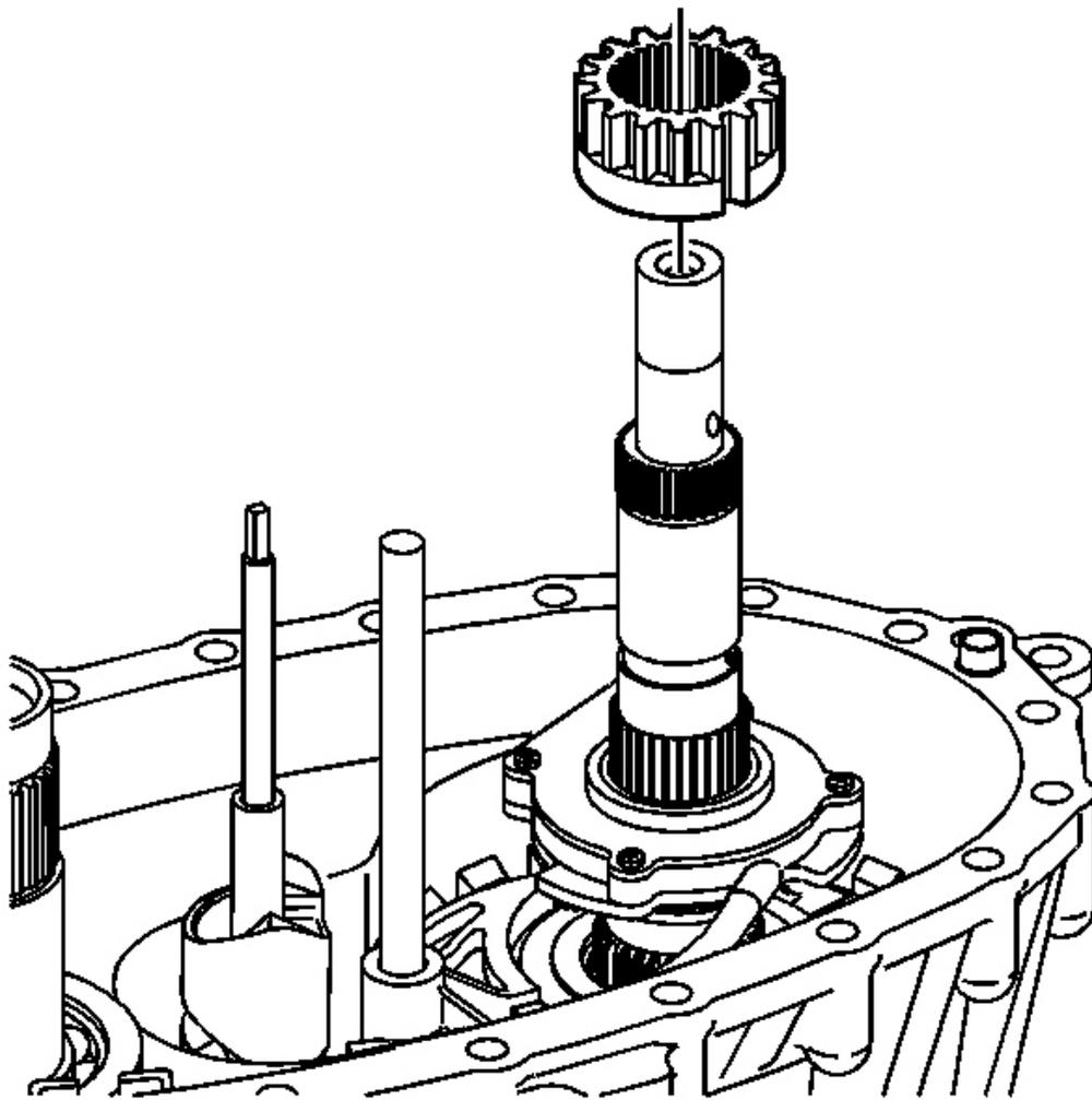
**Fig. 92: View Of Inner Lockup Hub**
