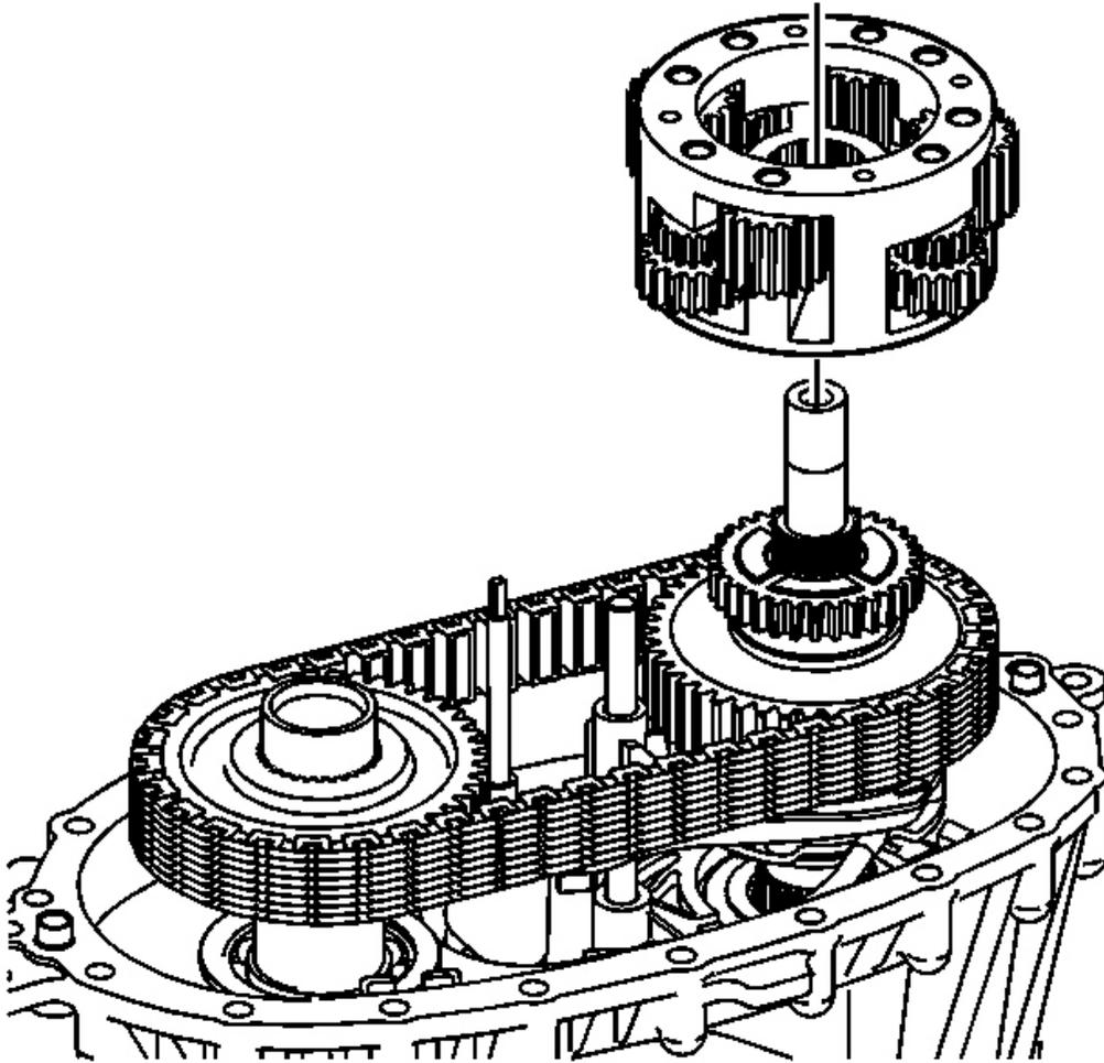
**Fig. 18: View Of Planetary Differential Assembly**
