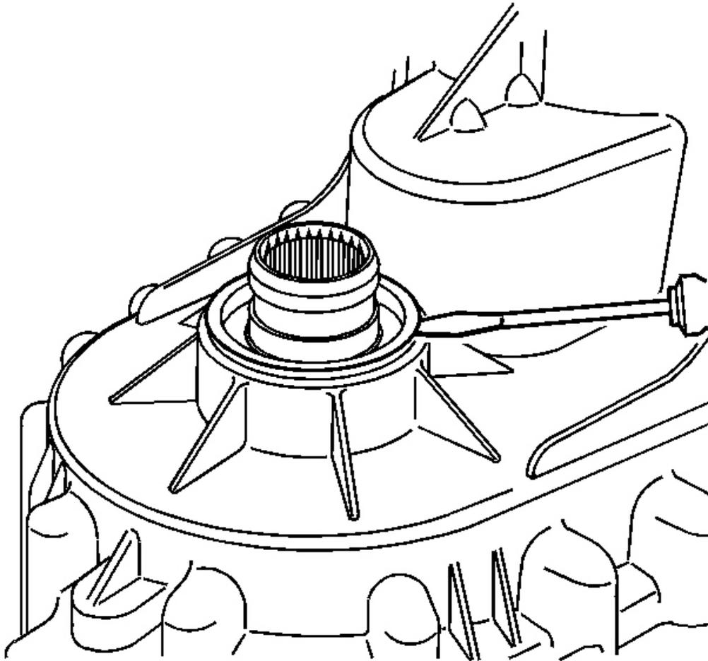
**Fig. 8: Locating Outer Lip Of The Front Output Shaft Seal**
