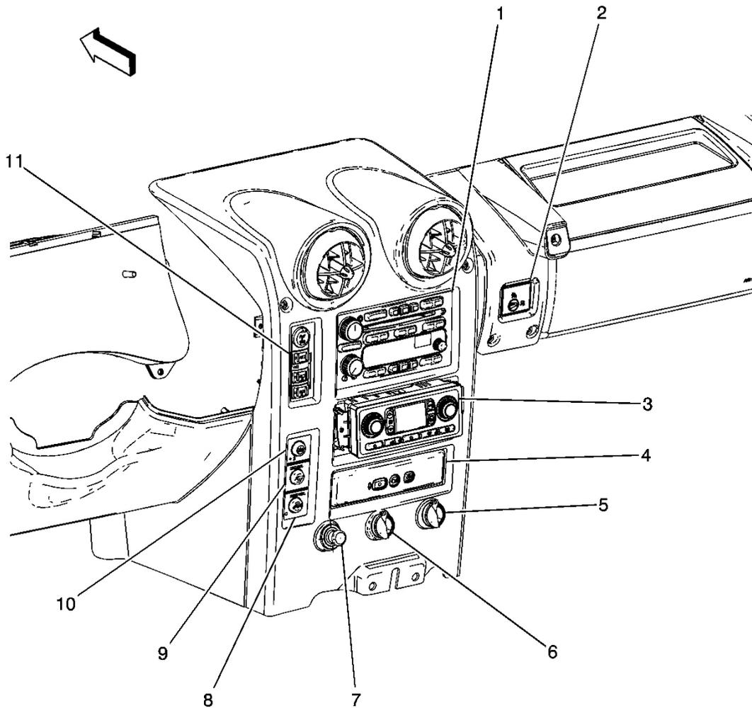
**Fig. 5: Center Of I/P Component Views**
