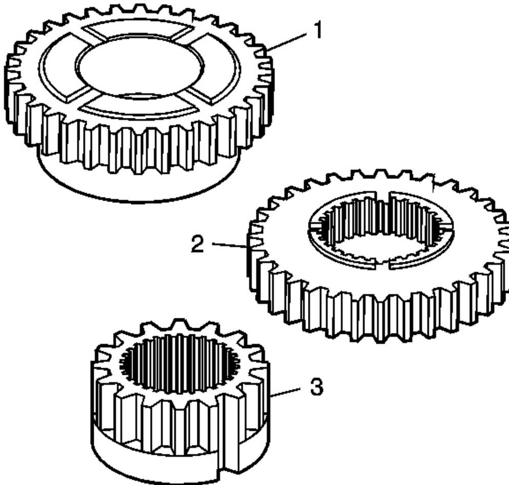
**Fig. 60: Identifying Front Sun Gear, Rear Sun Gear & Inner Lockup Hub**
