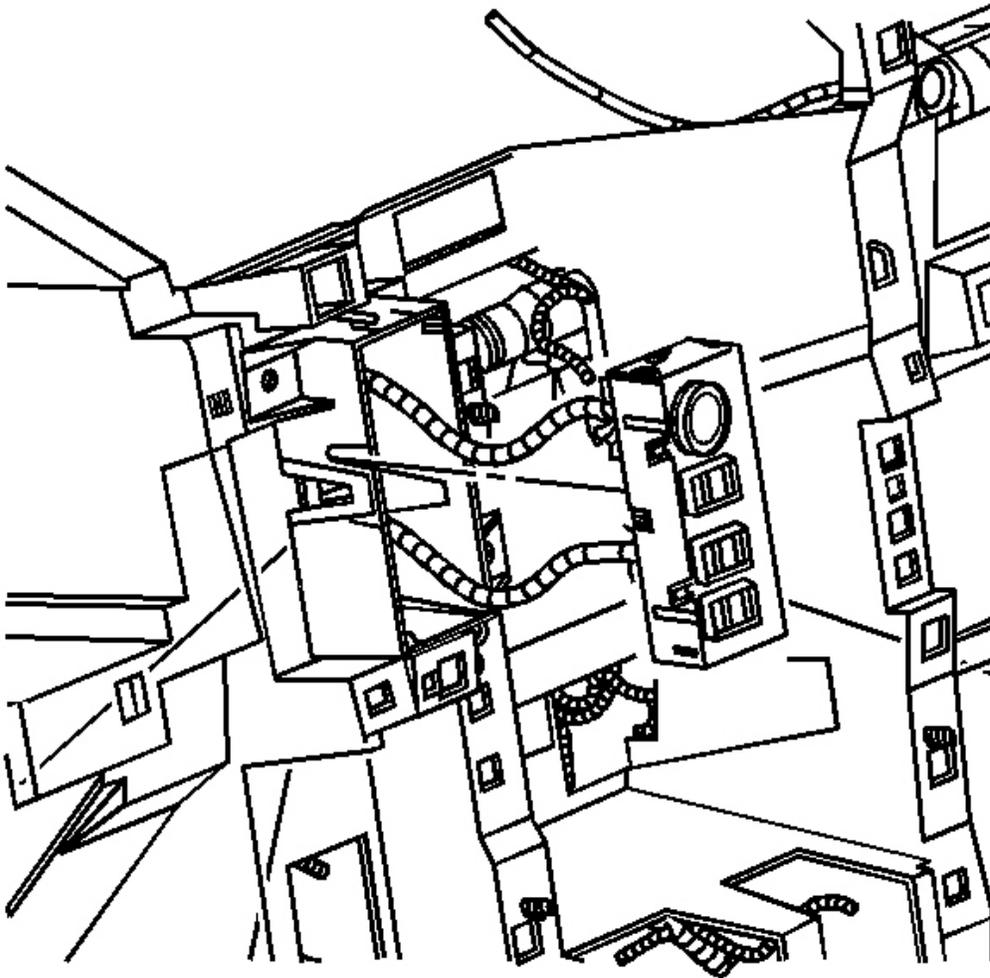
**Fig. 36: Shift Control/Selector Switch**
