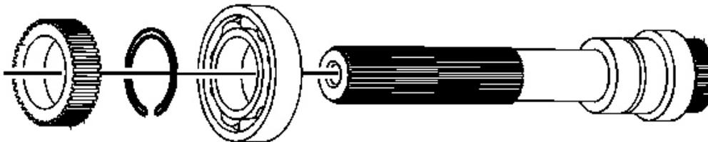
**Fig. 100: Rear Output Shaft**
