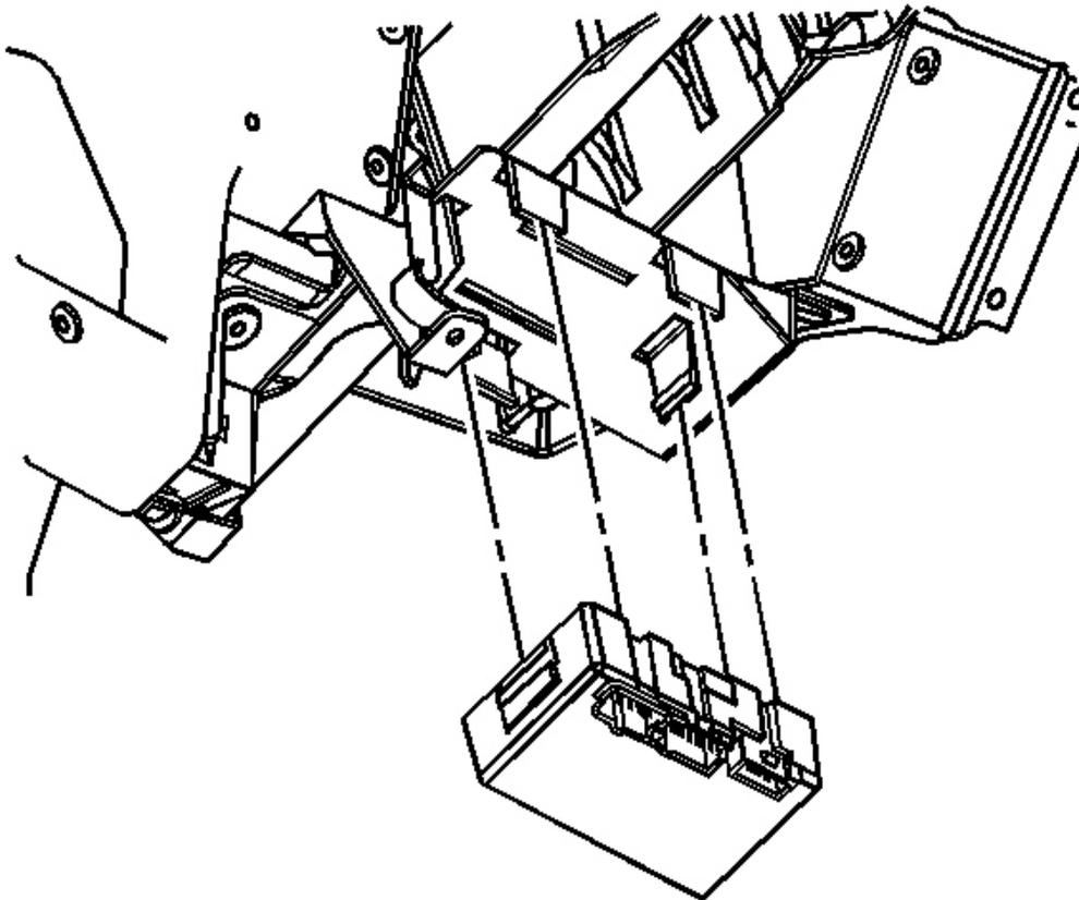
**Fig. 8: Transfer Case Shift Control Module**
