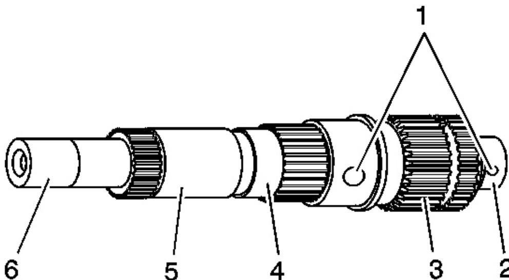
**Fig. 98: Front Support Bearing, Drive Gear Bushing, Front Sun Gear & Rear Support Bushing**
