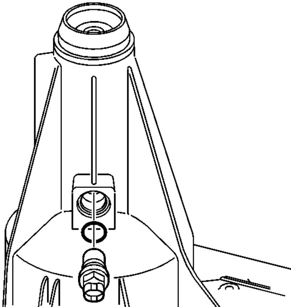
**Fig. 17: Speed Sensor & O-Ring**
