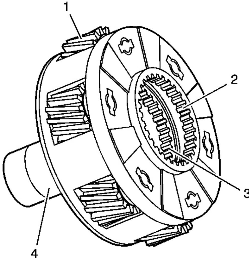
**Fig. 93: Inspecting High/Low Planetary Carrier**
