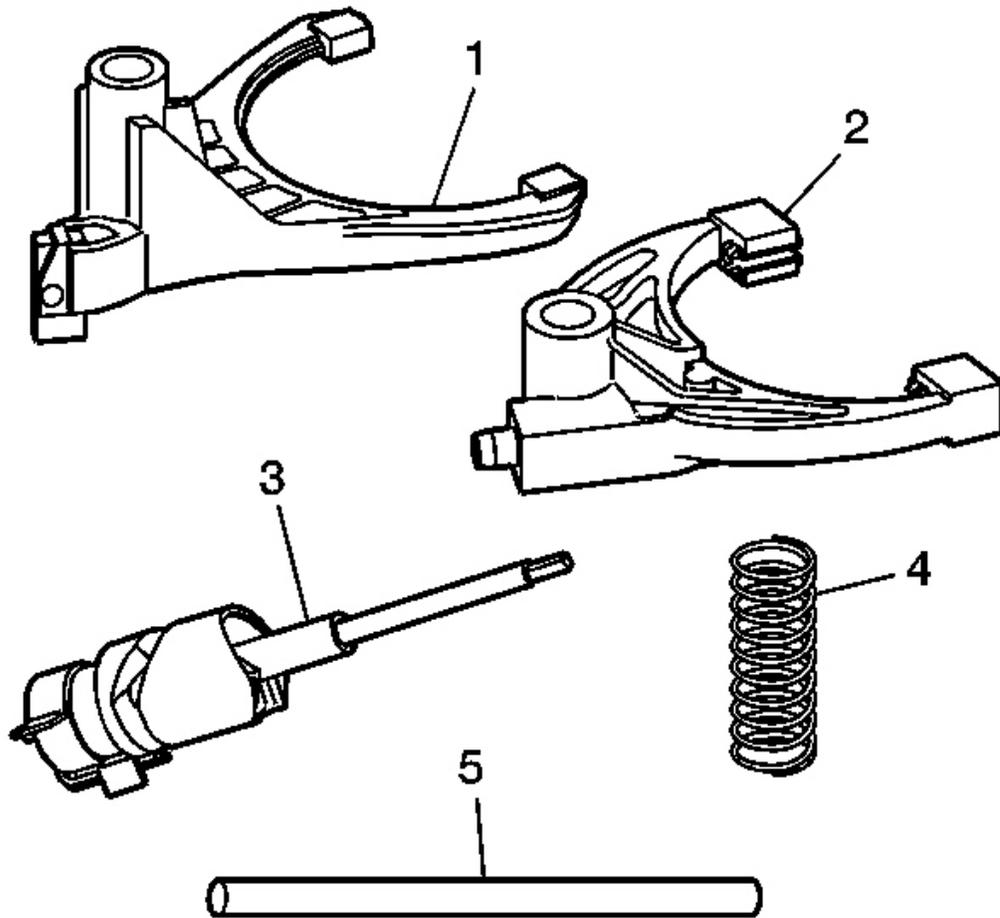
**Fig. 66: Identifying Shift System Components**
