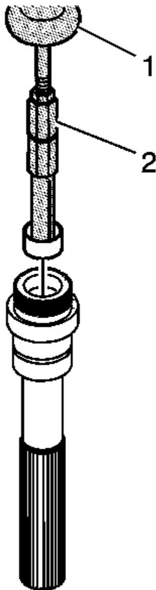
**Fig. 85: Removing Mainshaft Rear Support Bushing From Rear Output Shaft Using J 2619-01 & J 45548**
