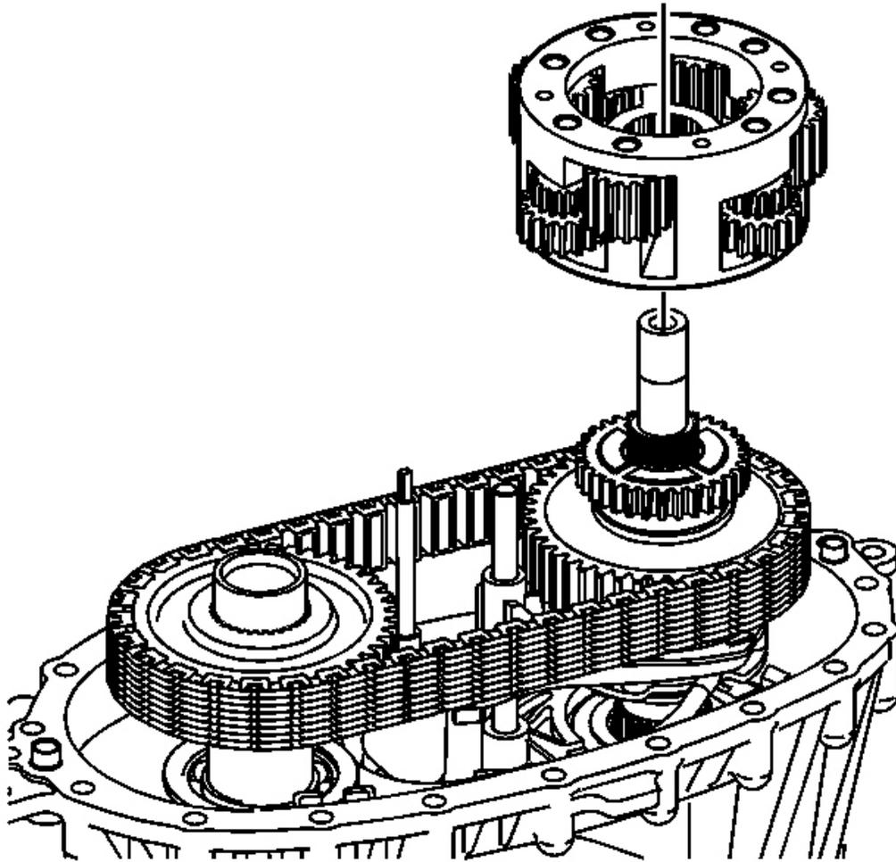
**Fig. 53: Planetary Differential Assembly**
