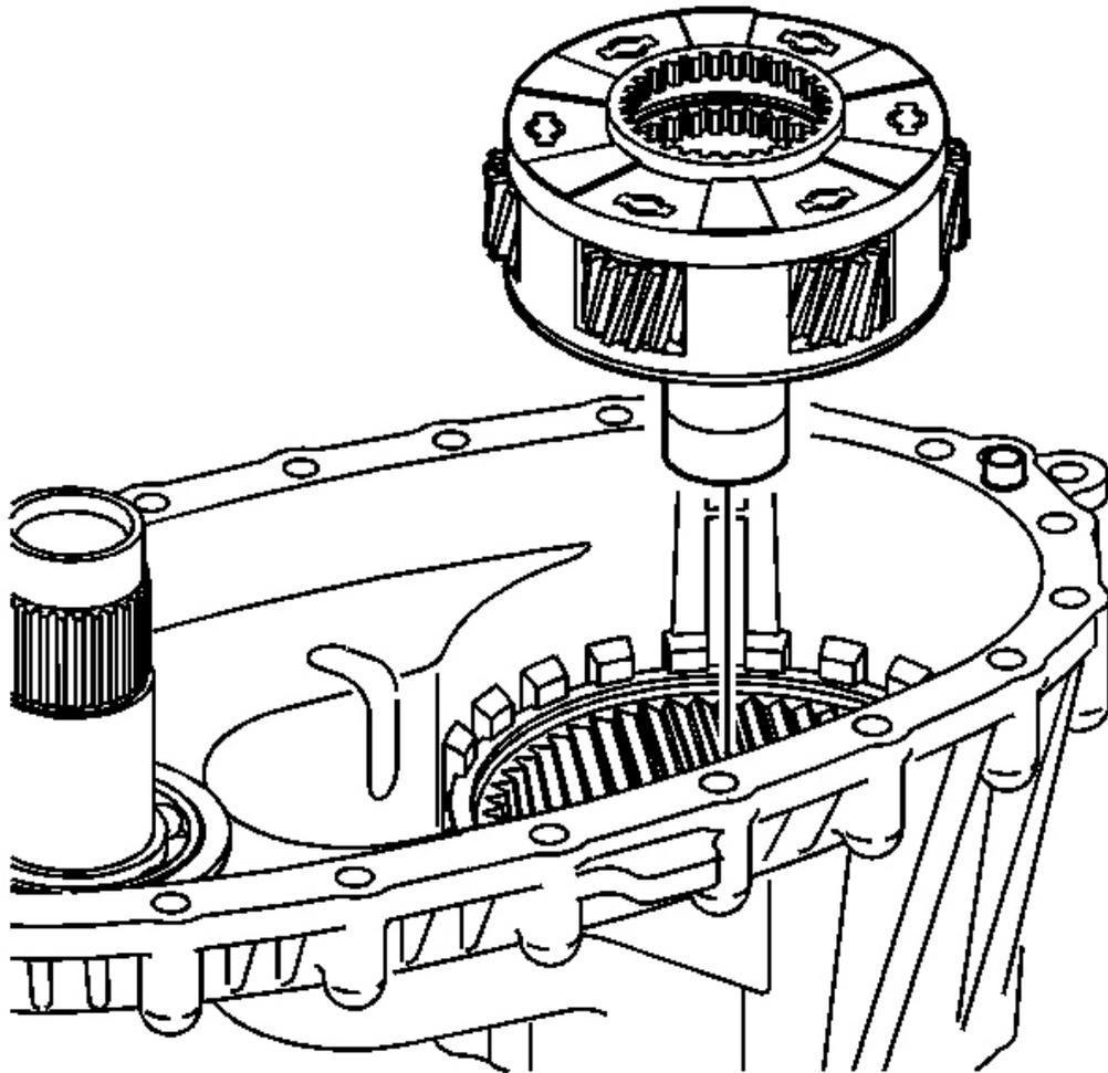
**Fig. 116: High/Low Planetary Carrier**
