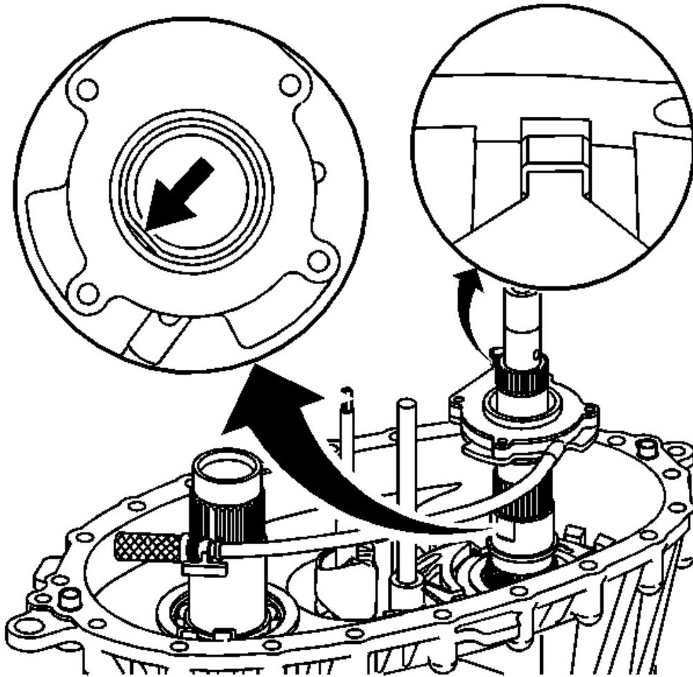
**Fig. 125: Oil Pump Assembly With Hose & Screen**
