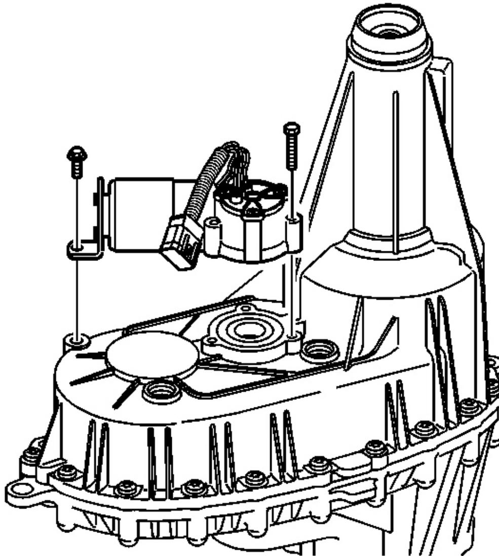
**Fig. 44: Transfer Case Encoder/Motor Assembly**
