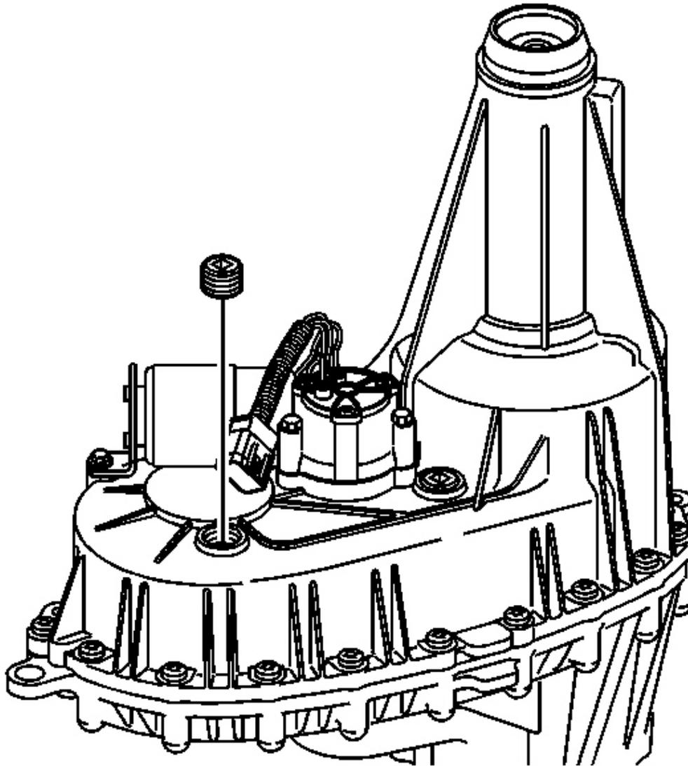
**Fig. 40: Drain Plug & Fill Plug**
