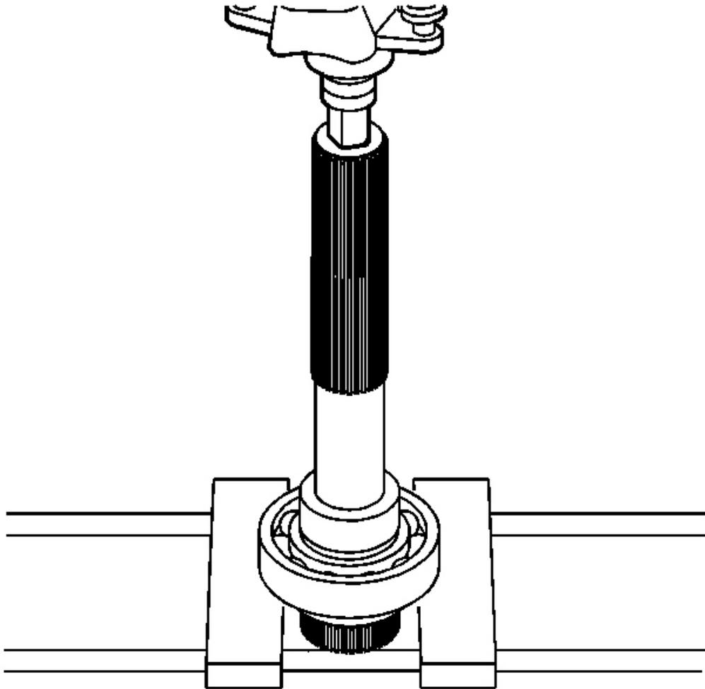
**Fig. 49: Pressing Out Rear Output Shaft Bearing**
