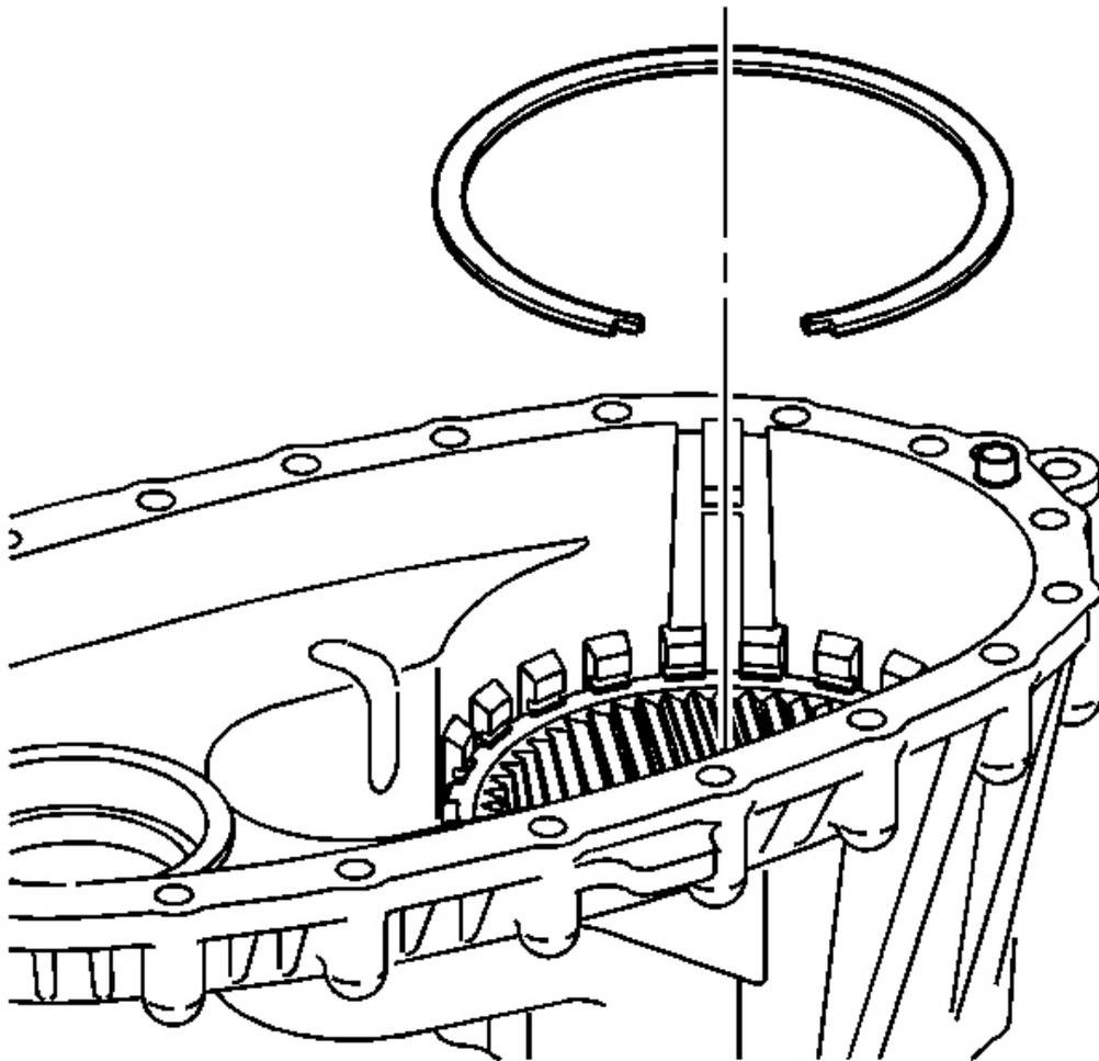
**Fig. 78: Retaining Ring & Annulus Gear**
