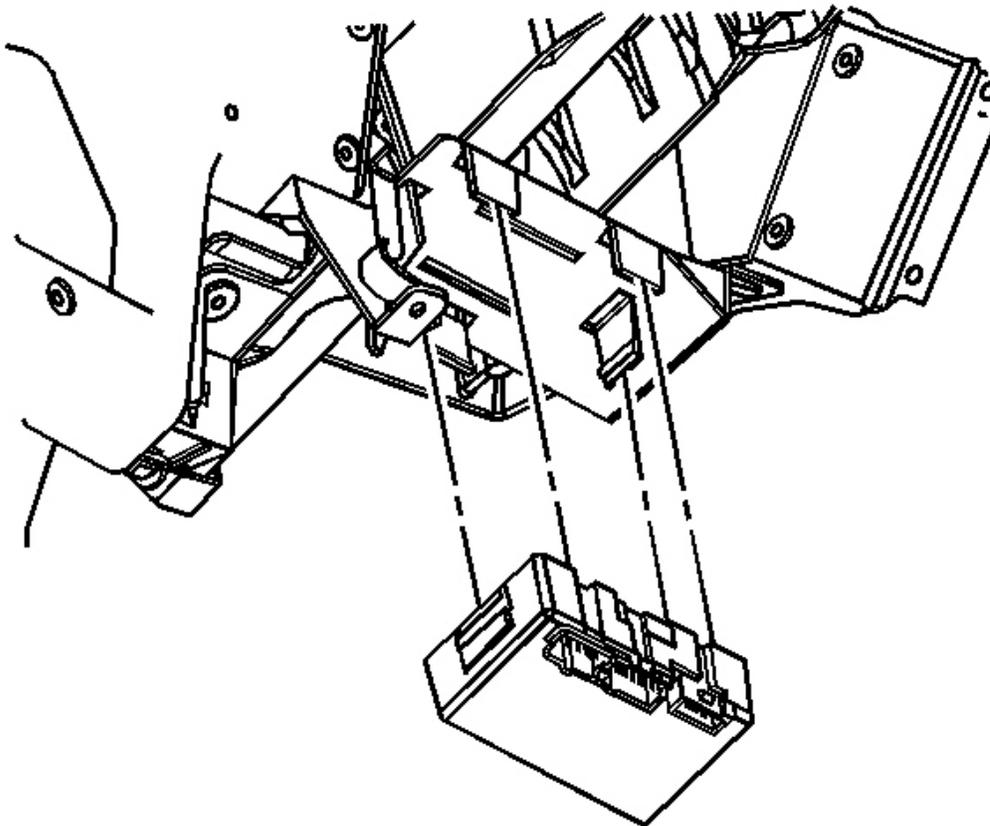
**Fig. 7: Transfer Case Shift Control Module**
