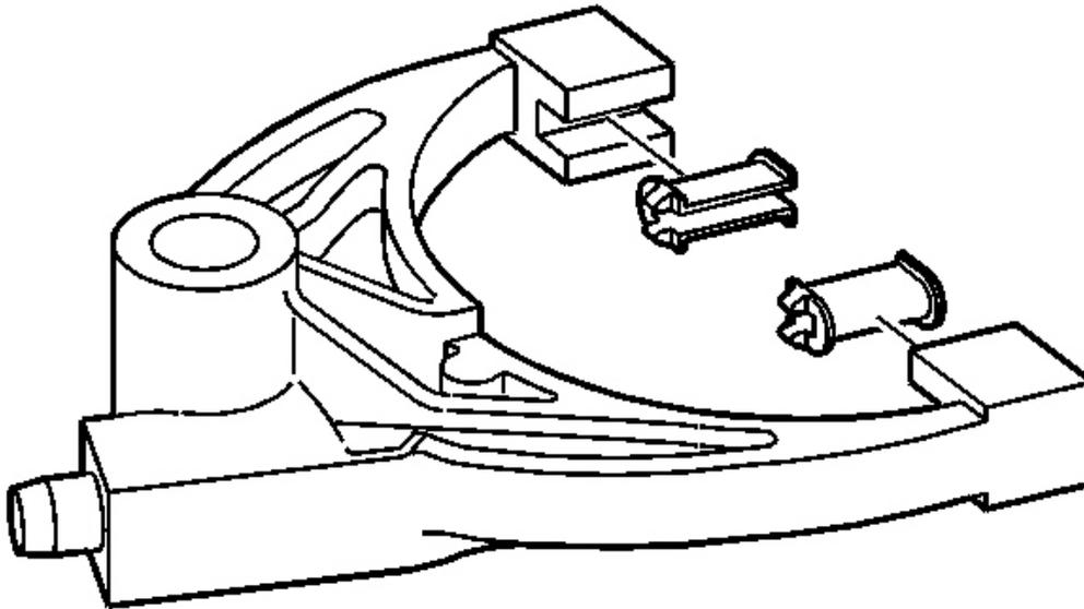
**Fig. 102: Inspecting Pads On High/Low Range Shift Fork For Wear**
