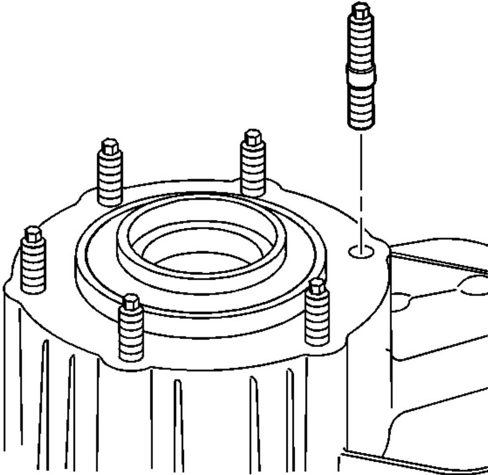
**Fig. 105: Installing Transfer Case Mounting Studs (If Removed)**
