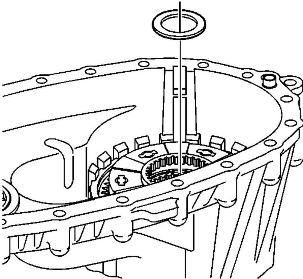
**Fig. 70: Input Shaft Thrust Washer**
