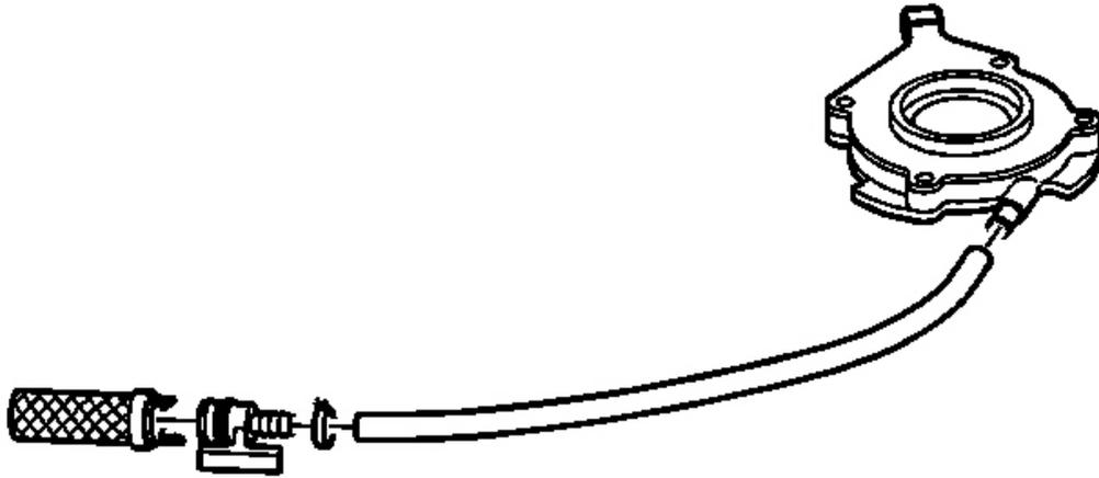
**Fig. 63: Oil Pump Hose & Oil Pump Screen**
