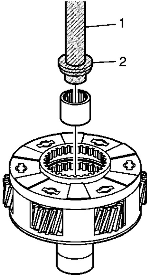
**Fig. 115: Installing Mainshaft Front Support Bearing Using J 42176 & J 45757**
