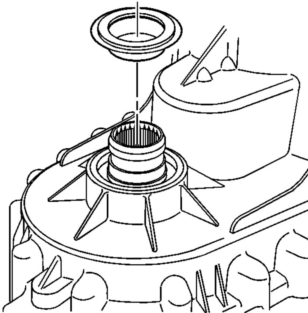
**Fig. 20: Inner Seal Race**
