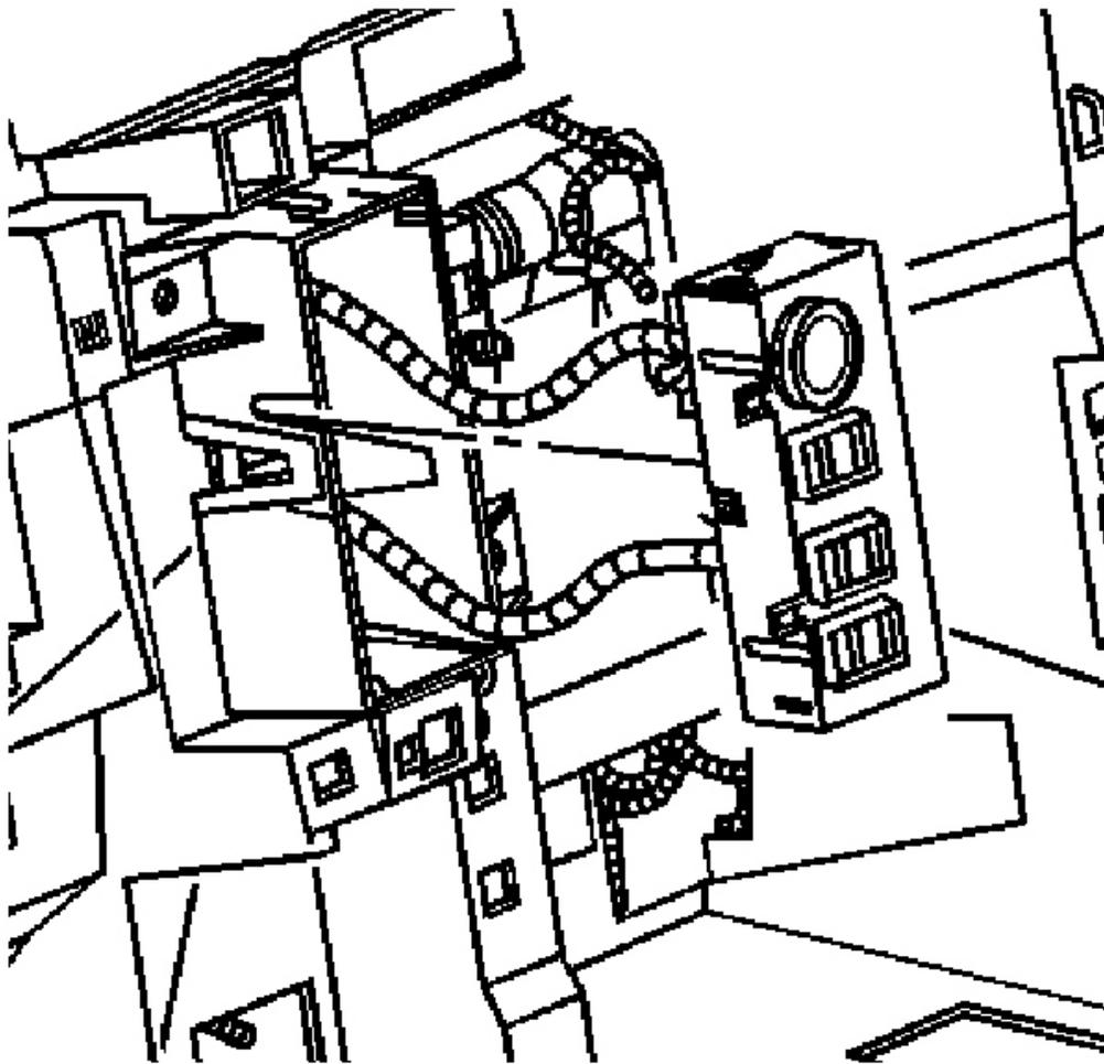
**Fig. 155: Transfer Case Shift Control Switch**
