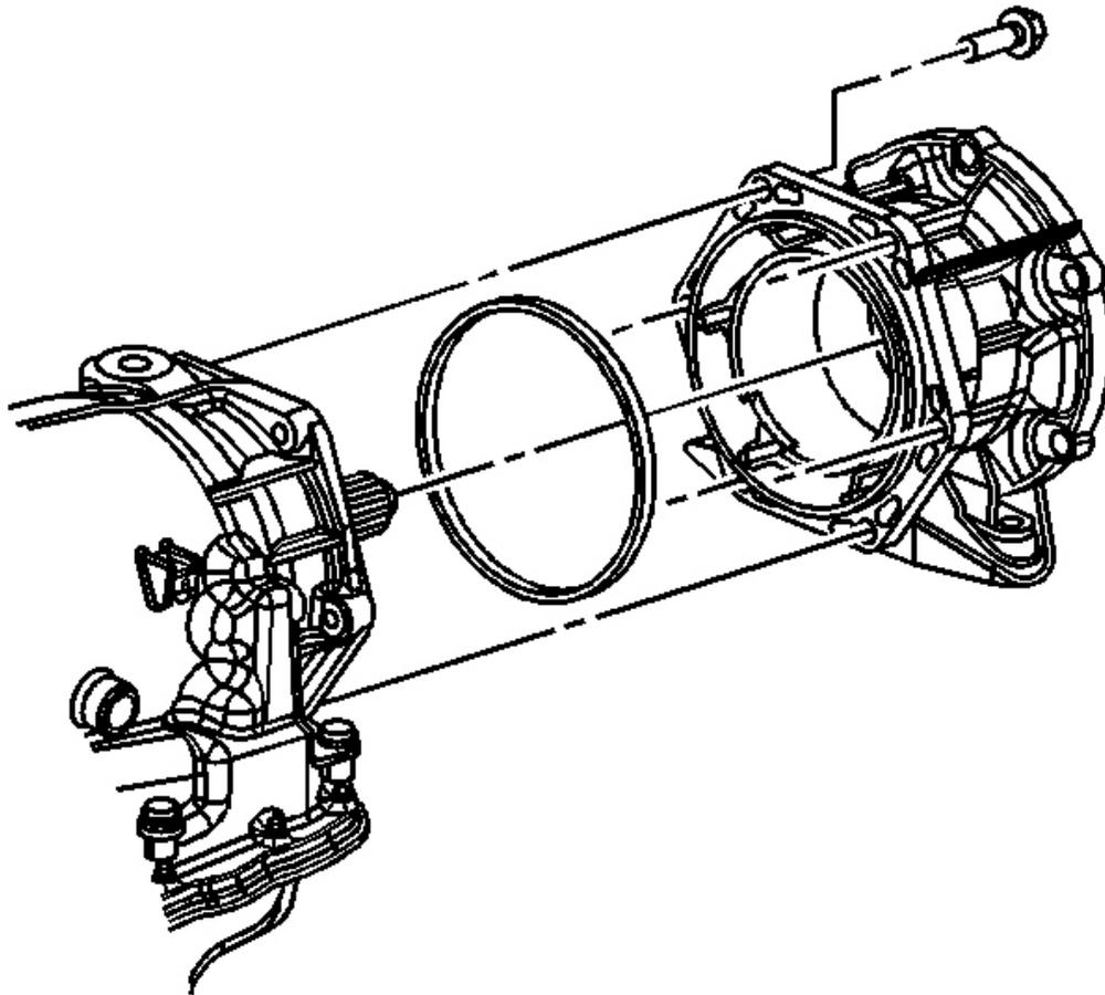
**Fig. 34: Transfer Case & Adapter**
