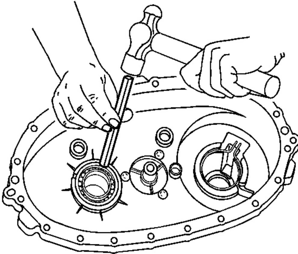
**Fig. 140: Installing Front Output Shaft Rear Bearing In Rear Case Half**
