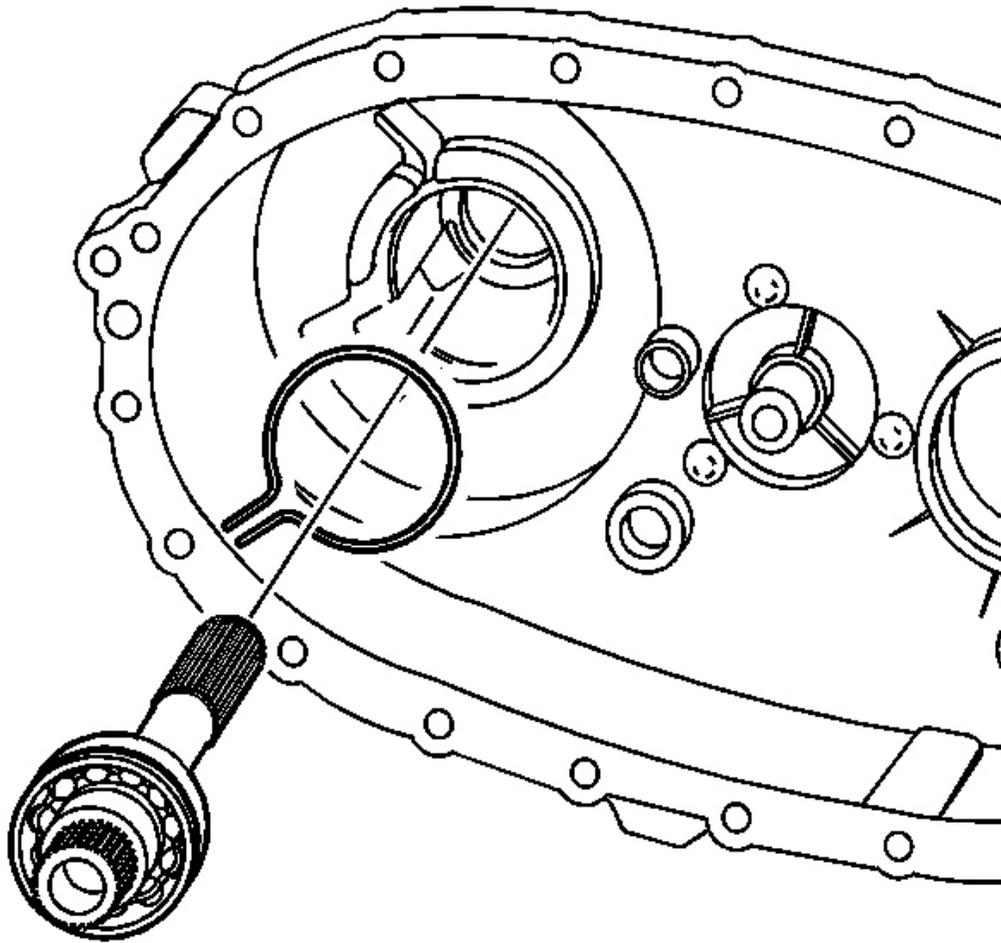
**Fig. 81: Rear Output Shaft & Rear Case Half**
