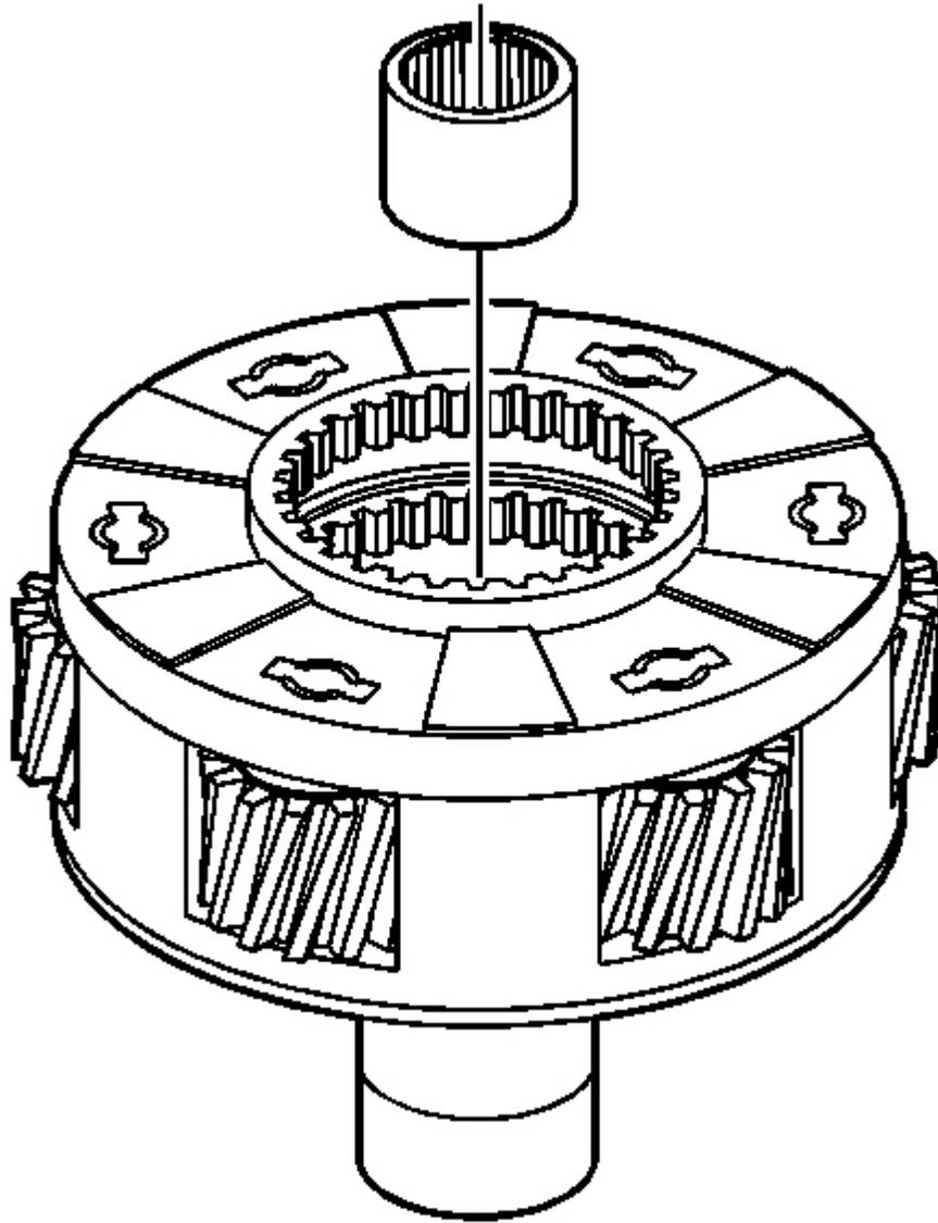
**Fig. 72: Inspecting Mainshaft Front Support Bearing**
