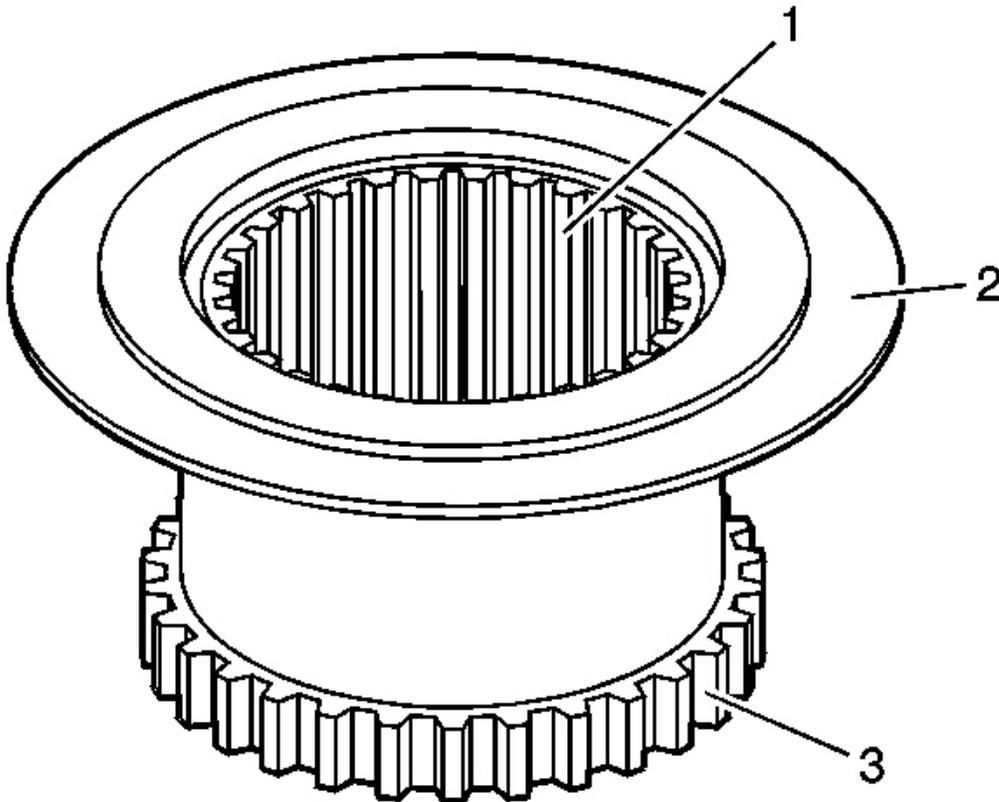
**Fig. 57: Identifying High/Low Range Shift Sleeve Inspection Areas**
