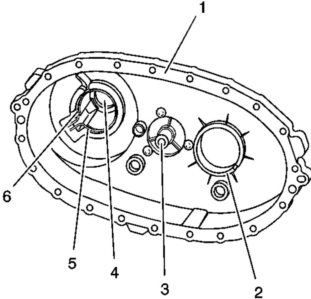
**Fig. 54: Locating Rear Case Half Inspection Points**
