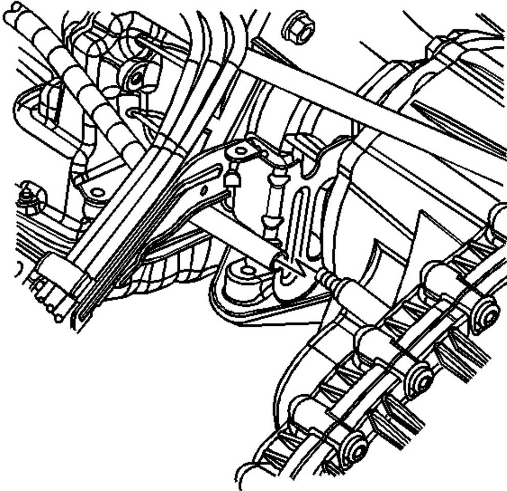
**Fig. 25: Removing Vent Hoses From Transfer Case & Transmission**
