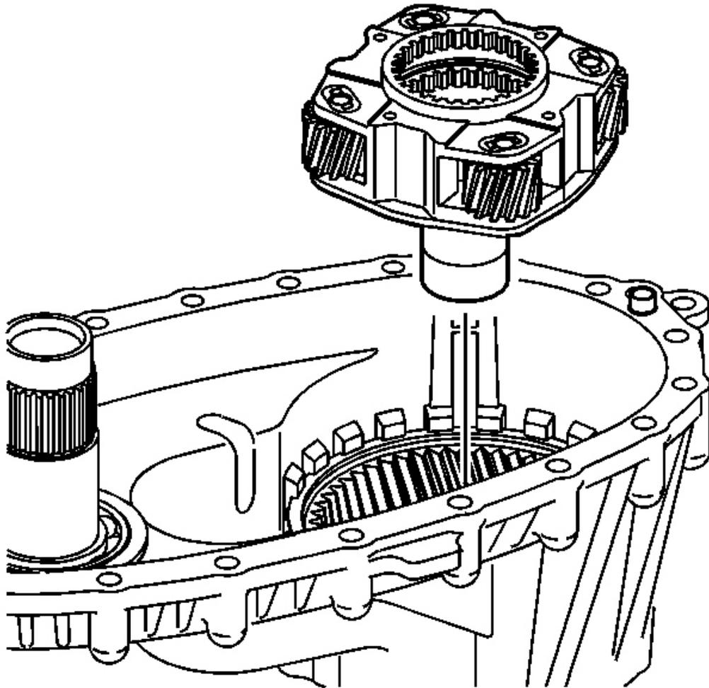
**Fig. 36: Identifying High/Low Planetary Carrier**
