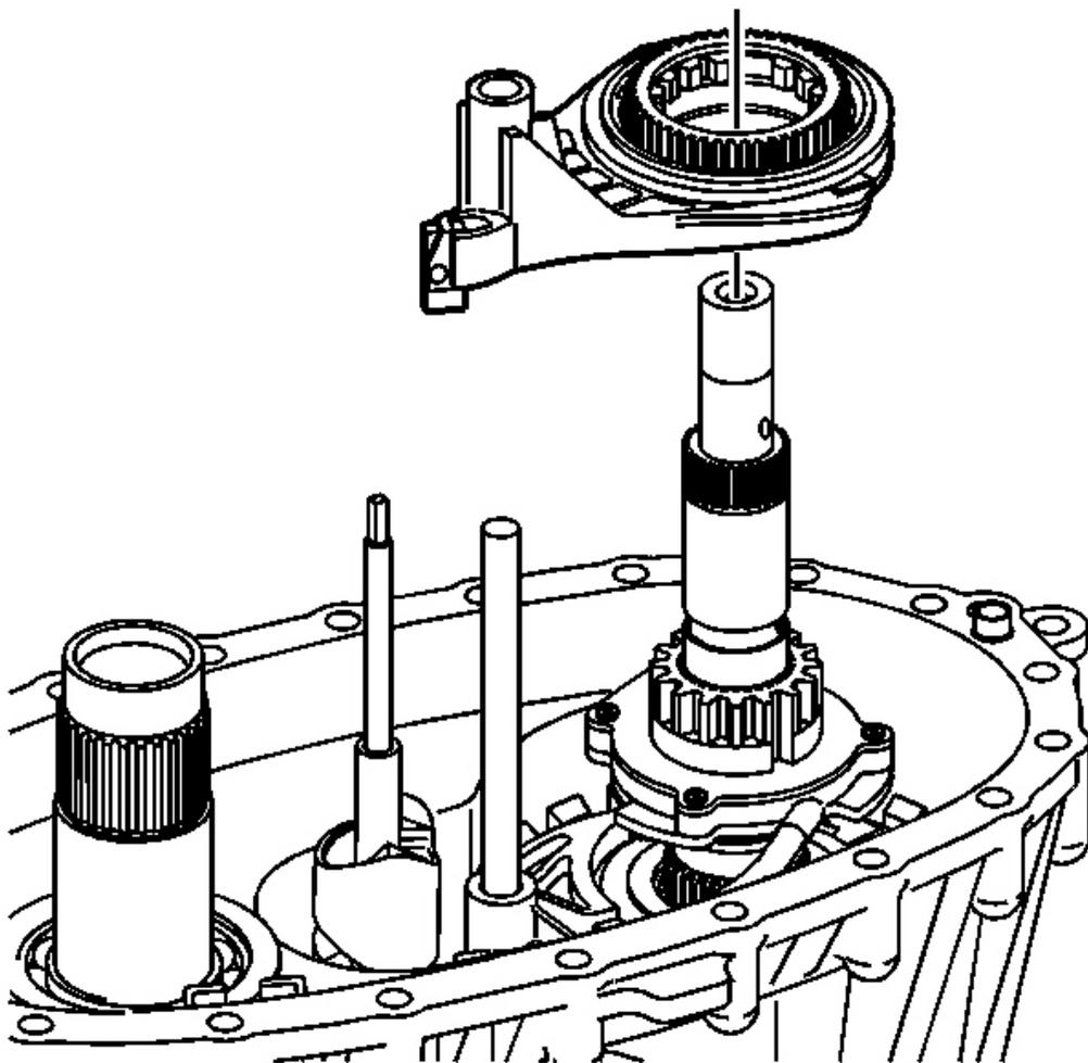
**Fig. 57: Lockup Shift Assembly & Lockup Mode Shift Fork**
