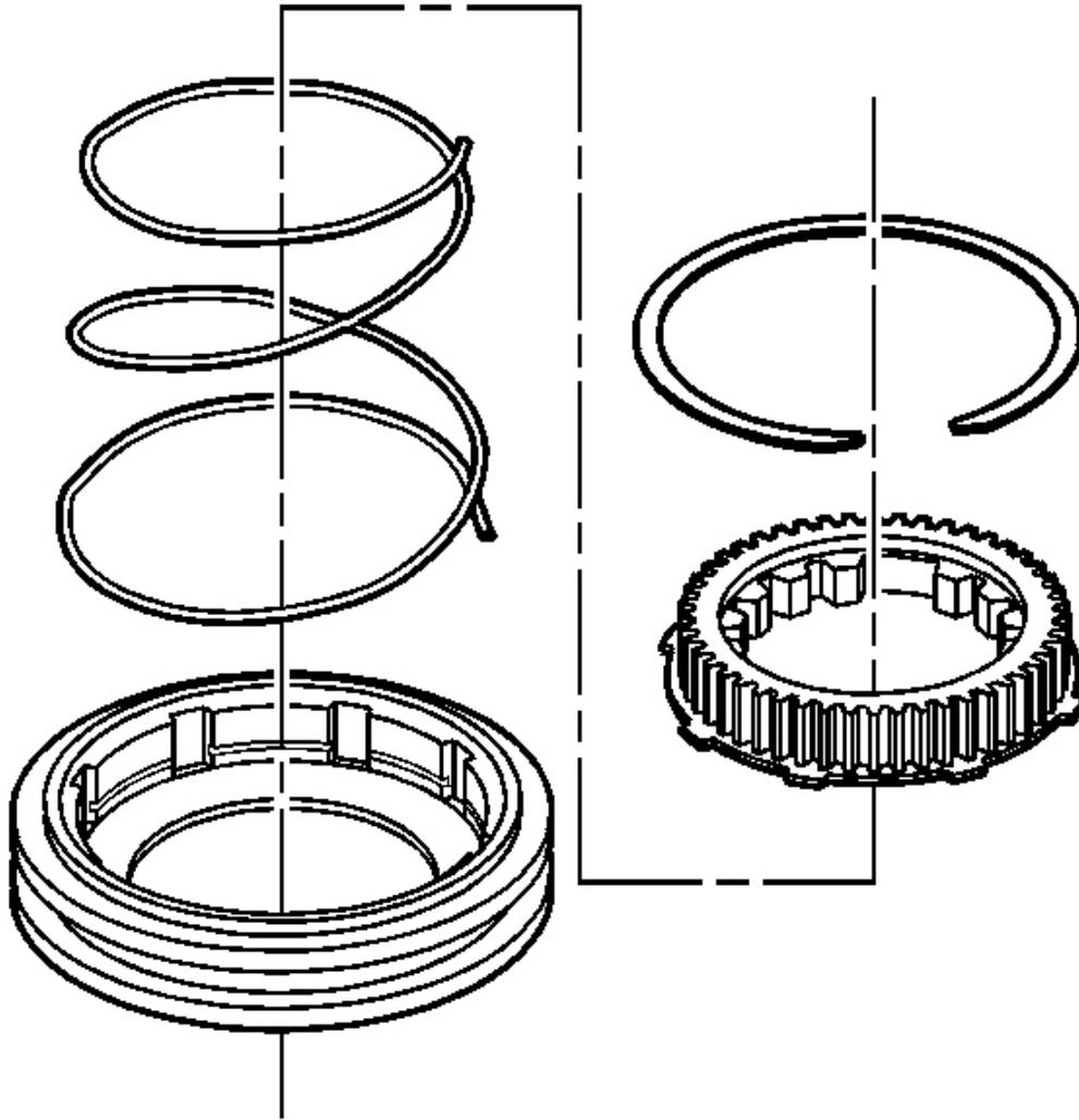
**Fig. 93: Illustrating Lockup Shift Assembly Components**
