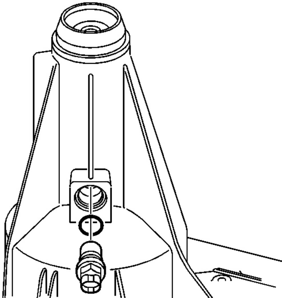
**Fig. 16: Speed Sensor & O-Ring**
