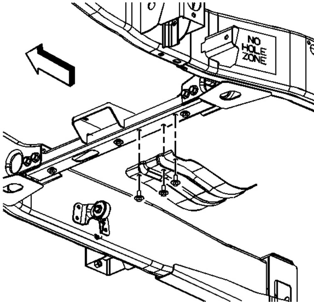
**Fig. 10: Transfer Case Shield**
