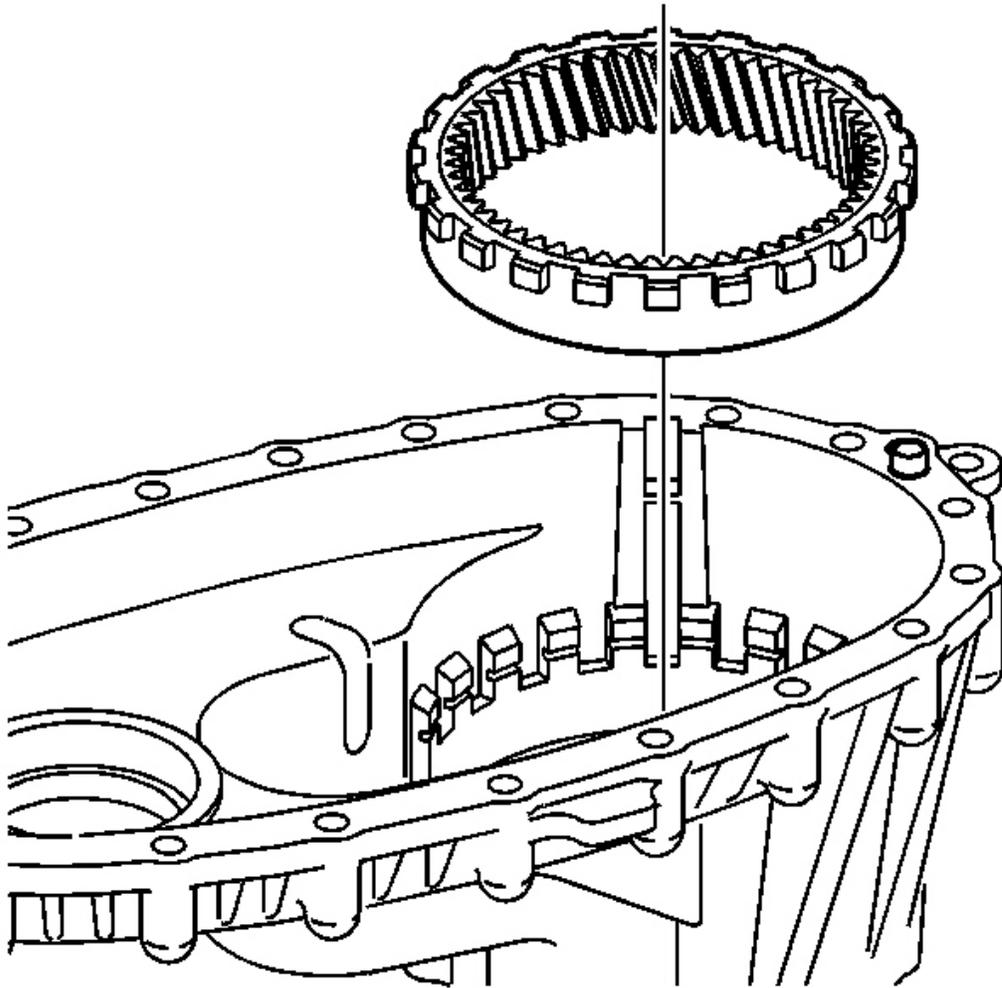
**Fig. 109: Annulus Gear & Front Case Half**
