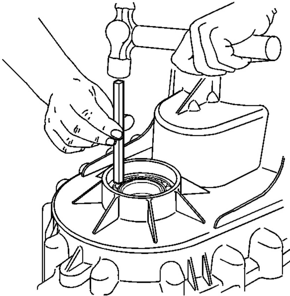
**Fig. 42: Removing Front Output Shaft Bearing**
