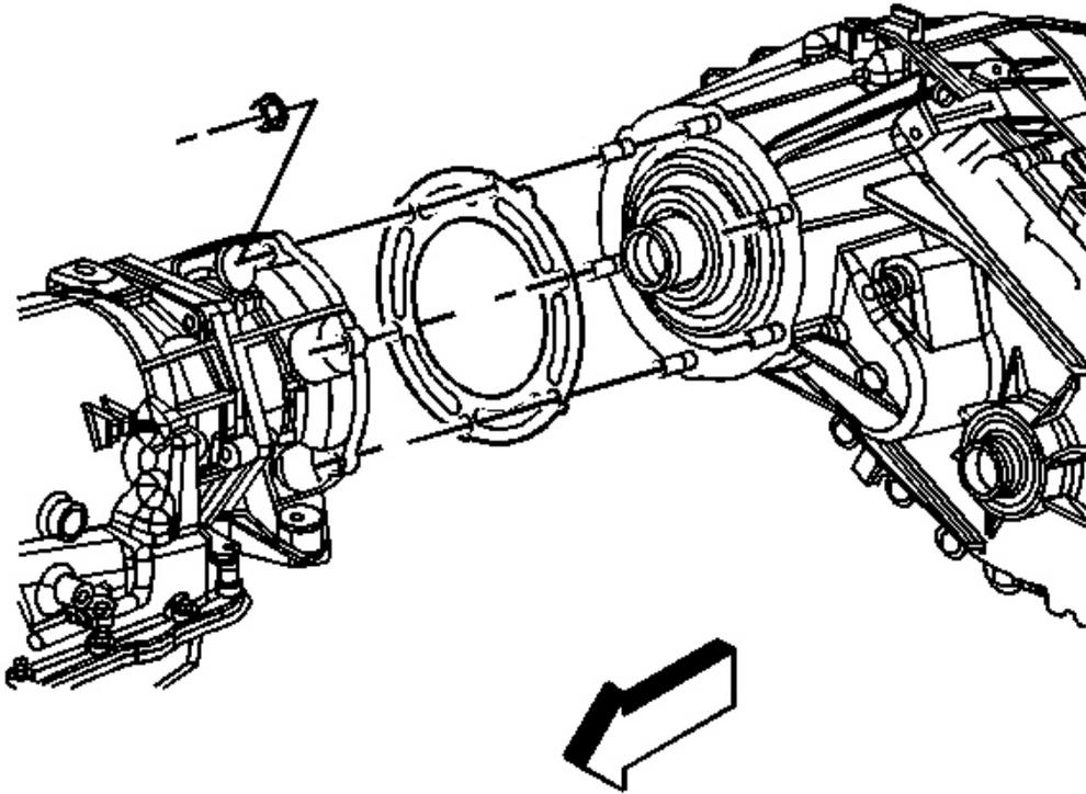
**Fig. 28: Transfer Case Assembly**
