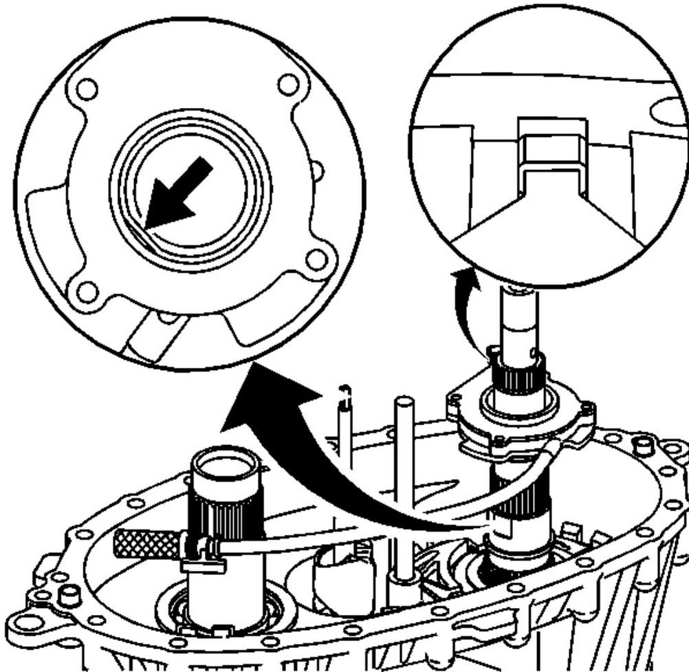
**Fig. 62: Oil Pump Assembly With Hose & Screen**
