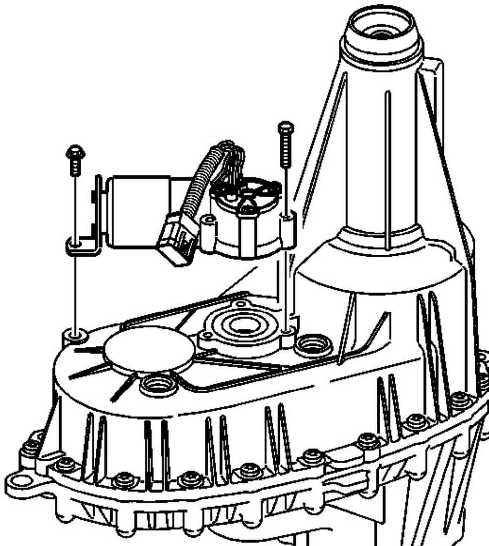
**Fig. 14: Transfer Case Encoder/Motor Assembly**
