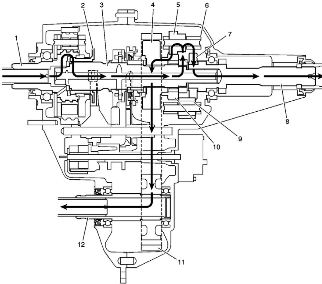
**Fig. 156: 4HI Mode Power Flow**
