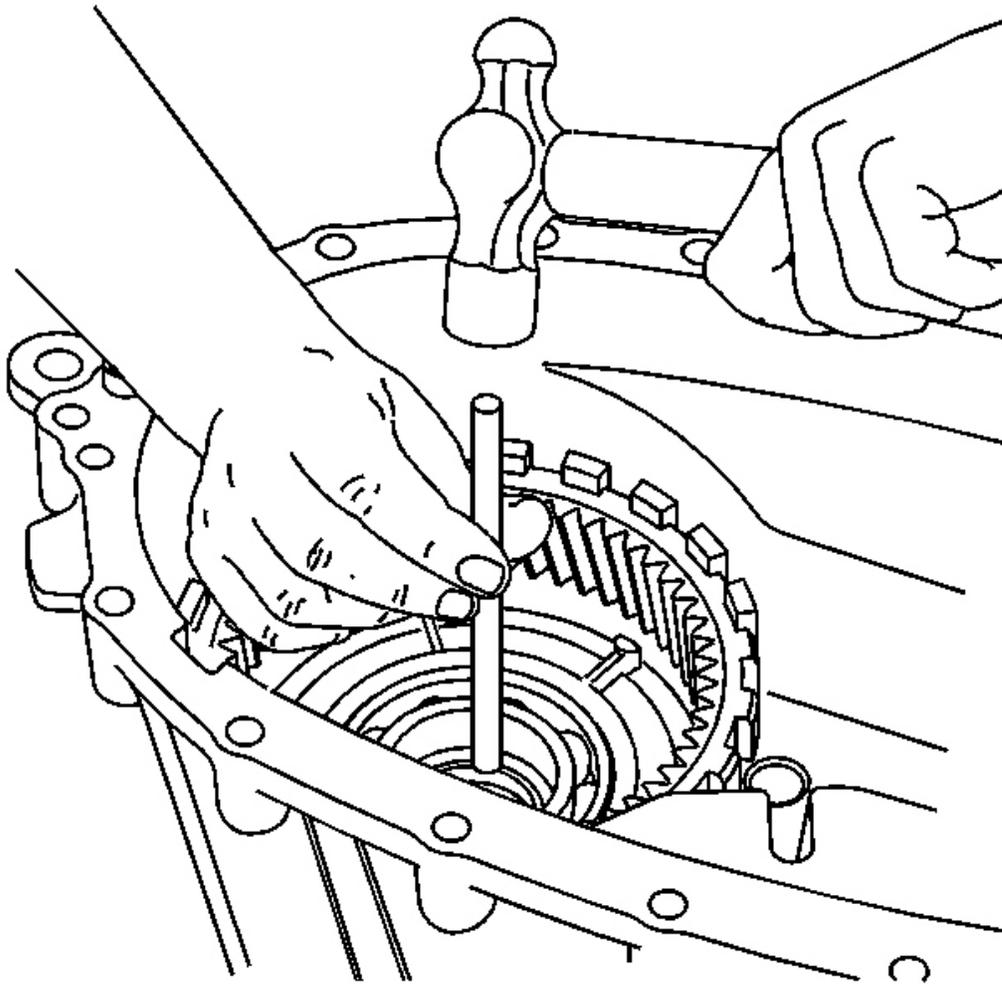
**Fig. 75: Removing Input Seal By Using Hammer & Punch**
