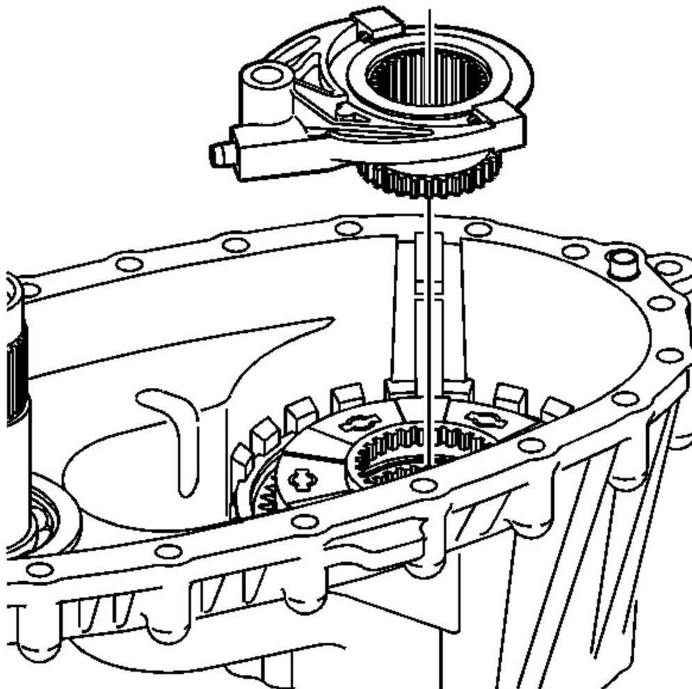
**Fig. 68: High/Low Range Sleeve & High/Low Range Shift Fork**
