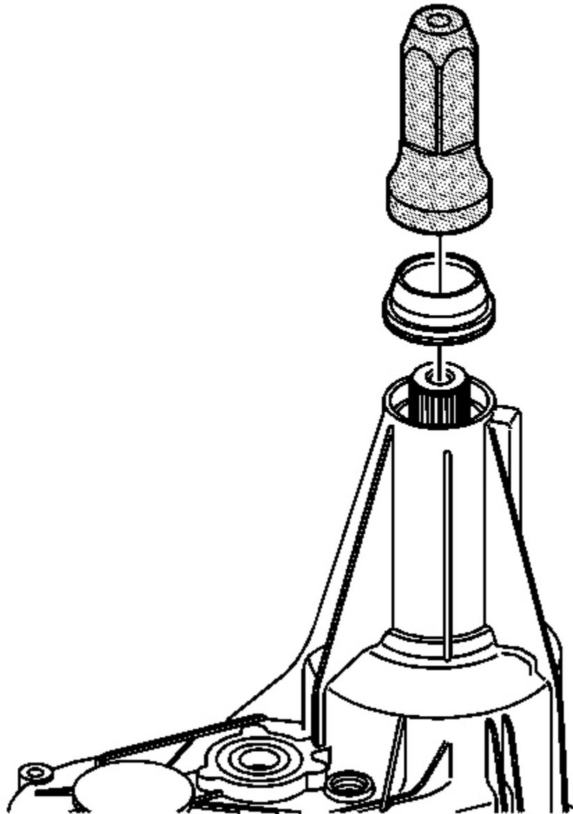
**Fig. 24: Using J 45756 To Install NEW Front Output Shaft Seal**
