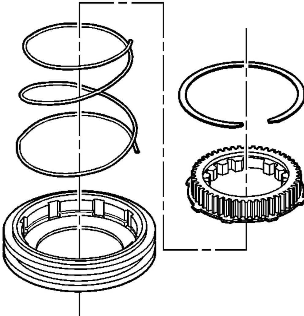
**Fig. 96: Lockup Shift Assembly**
