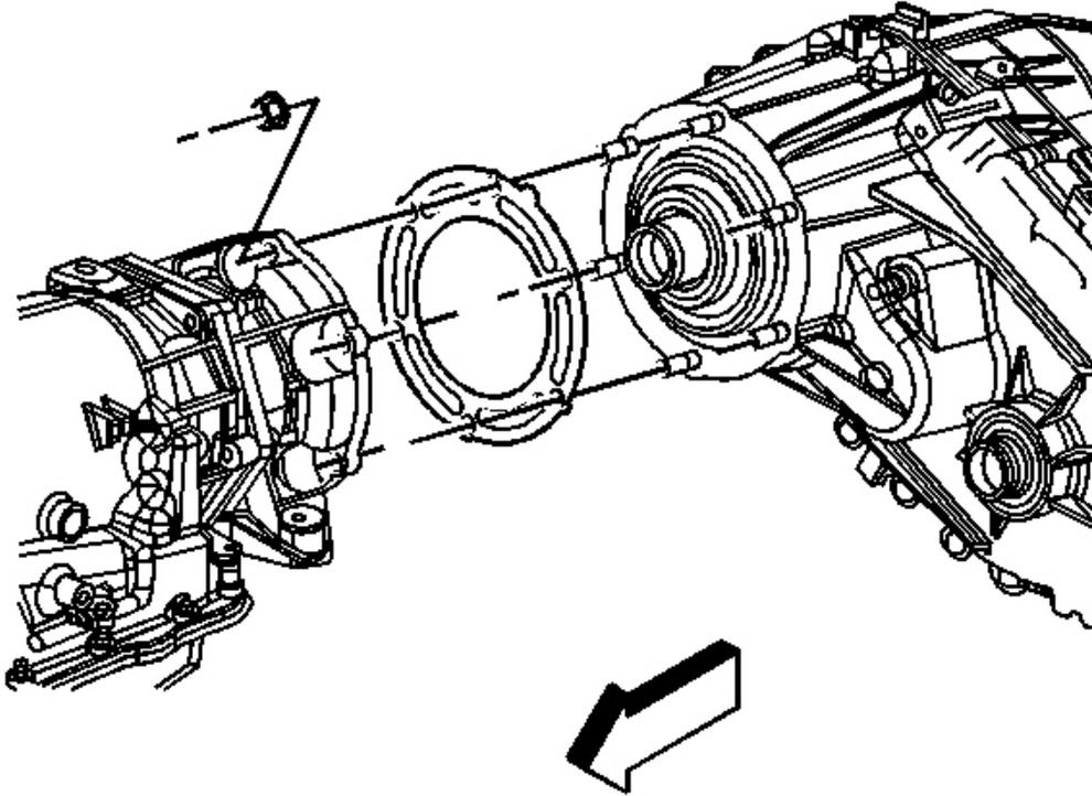
**Fig. 27: Transfer Case Assembly**
