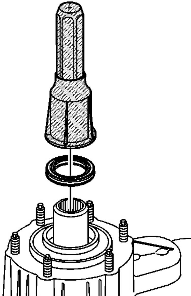
**Fig. 154: Installing Front Input Shaft Seal By Using J 42738**
