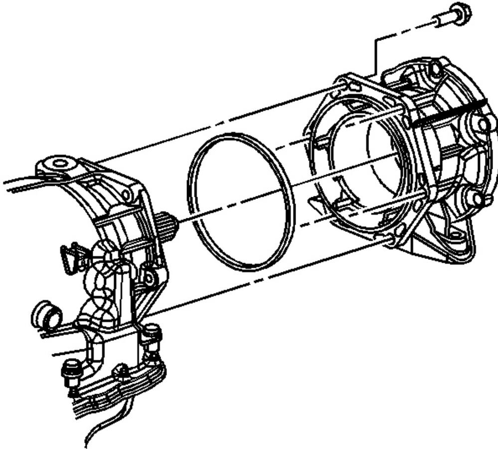
**Fig. 33: Transfer Case & Adapter**
