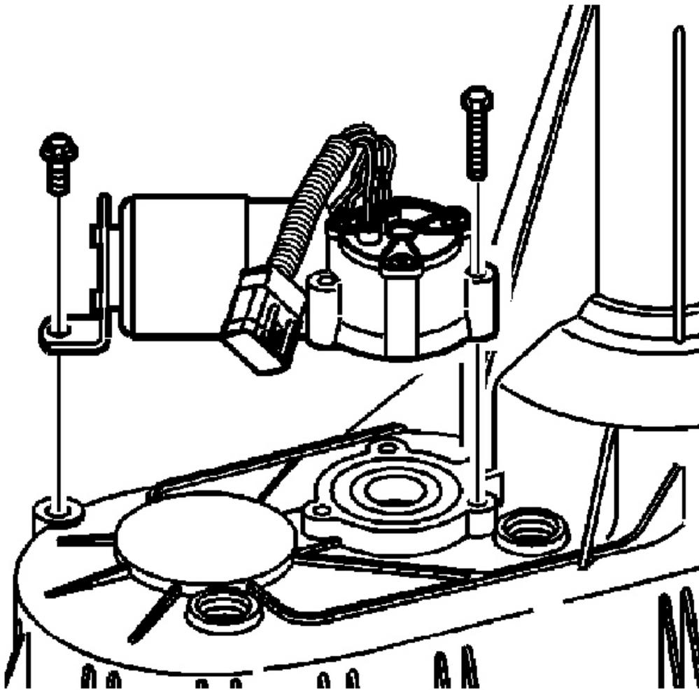
**Fig. 159: Transfer Case Encoder Motor**
