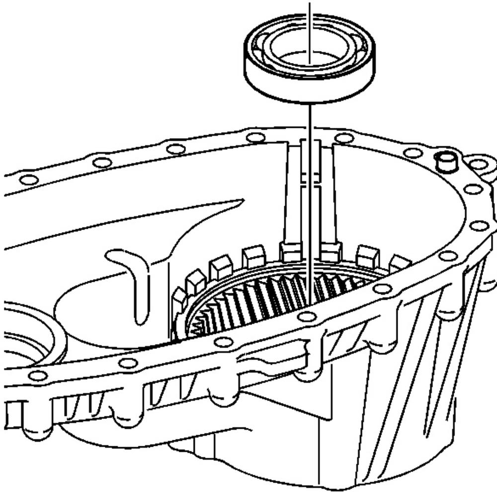
**Fig. 76: Installing Input Shaft Bearing**
