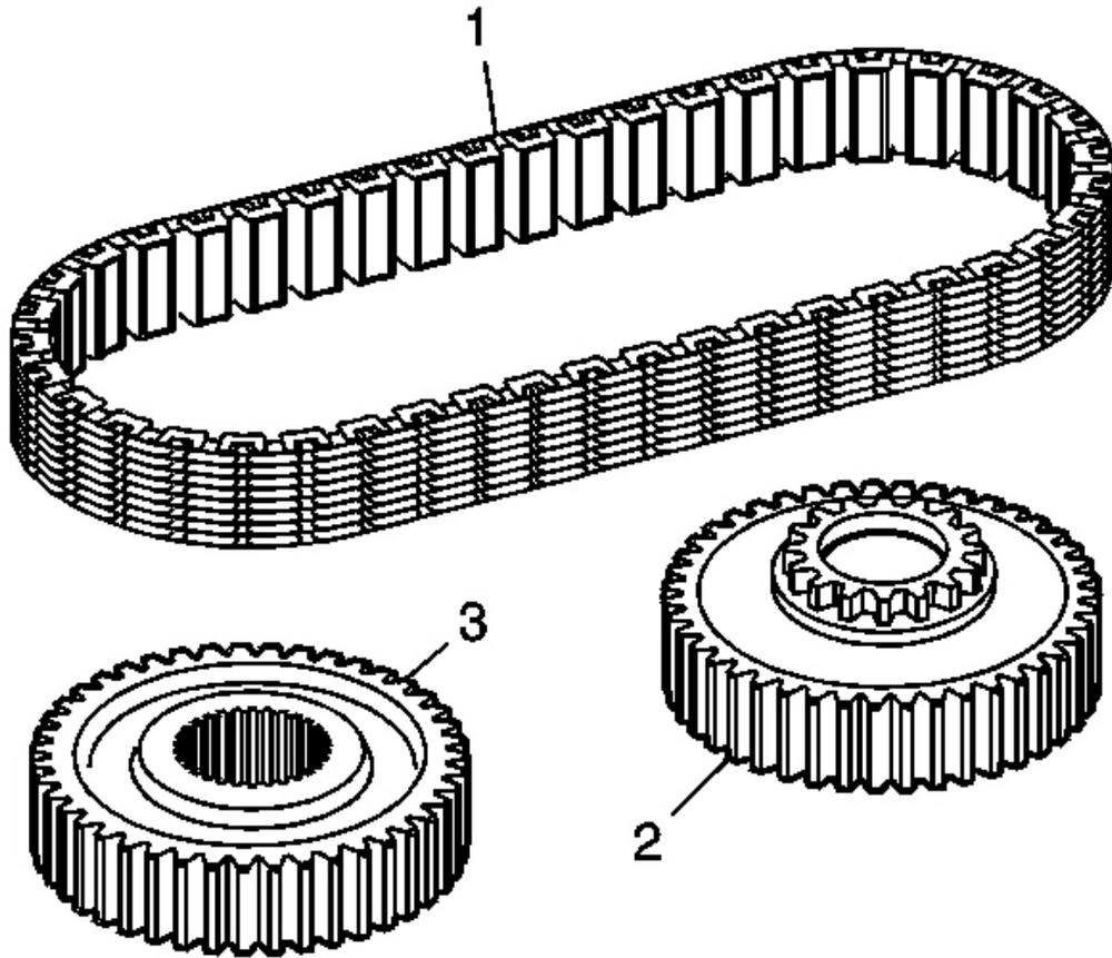
**Fig. 97: Drive Chain, Drive Sprocket & Driven Sprocket**
