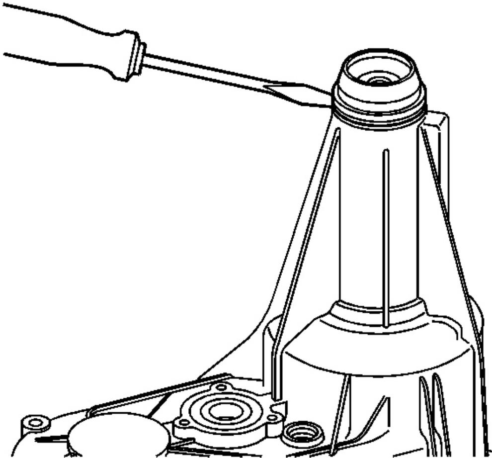
**Fig. 11: Removing Rear Output Shaft Seal**
