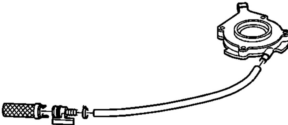
**Fig. 90: Oil Pump Hose & Oil Pump Screen**
