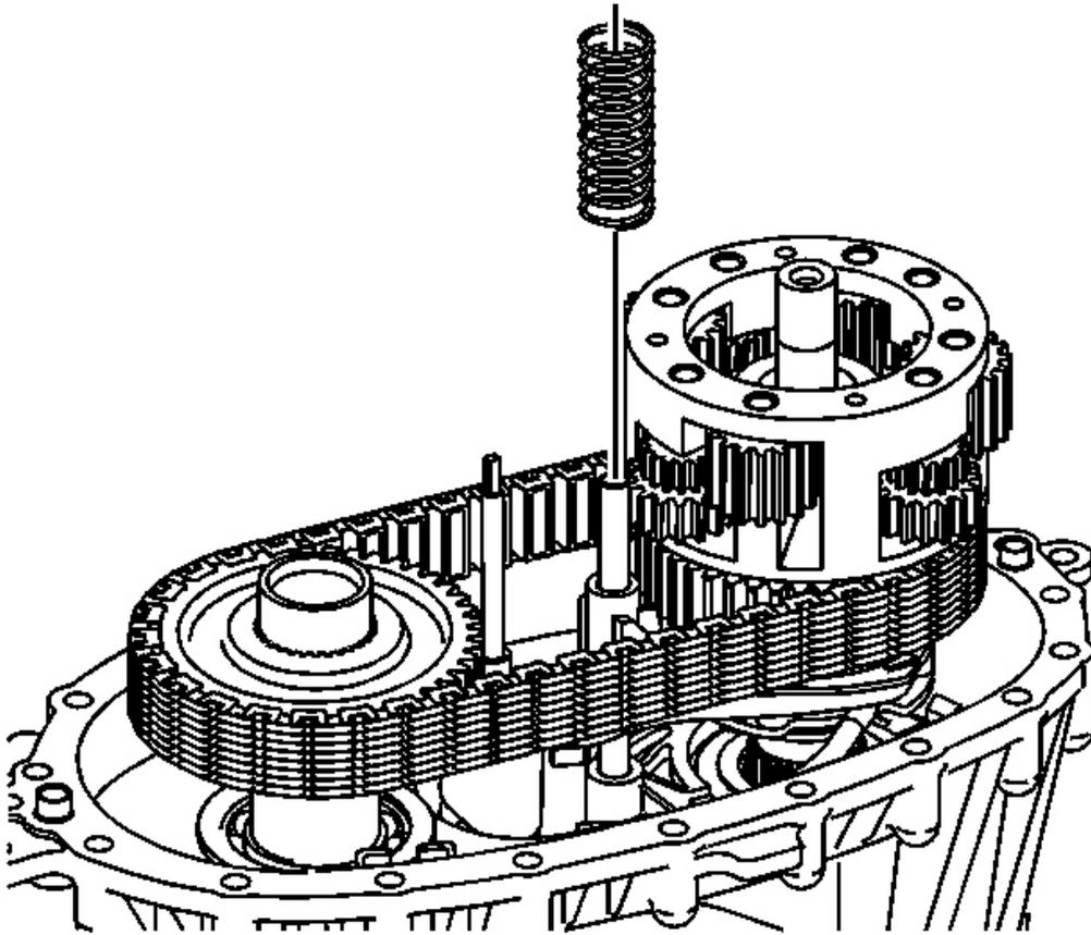
**Fig. 104: Identifying Shift Fork Shaft Spring**
