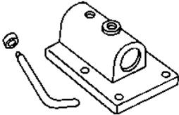
A holding fixture with a rectangular base, a central cylindrical opening, and a curved arm extending from the side.       | J 3289-20<br>Holding Fixture                       |
