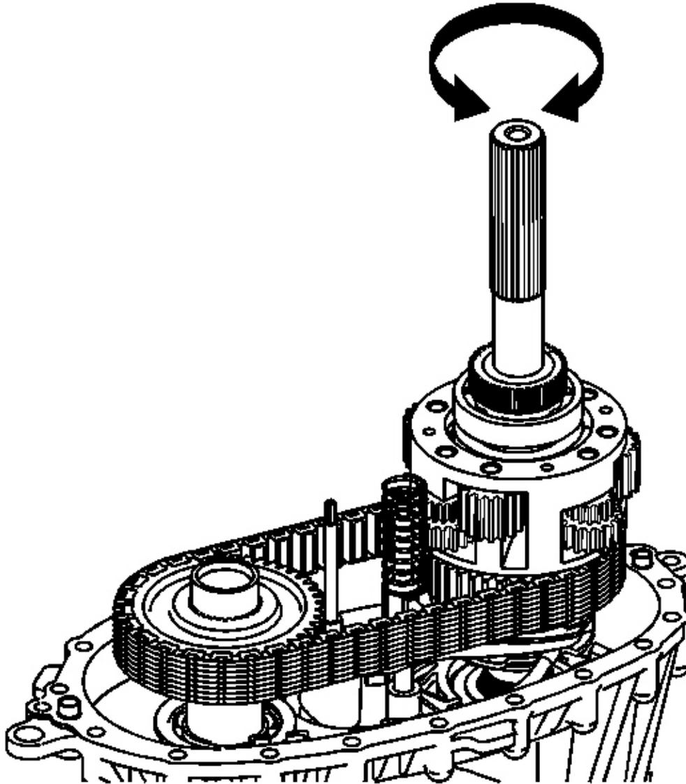
**Fig. 103: Checking Planetary Differential Pinion Gear Rotation With Rear Output Shaft**
