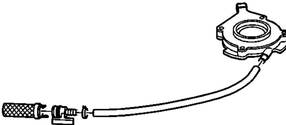
**Fig. 55: Locating Oil Pump Hose & Screen**
