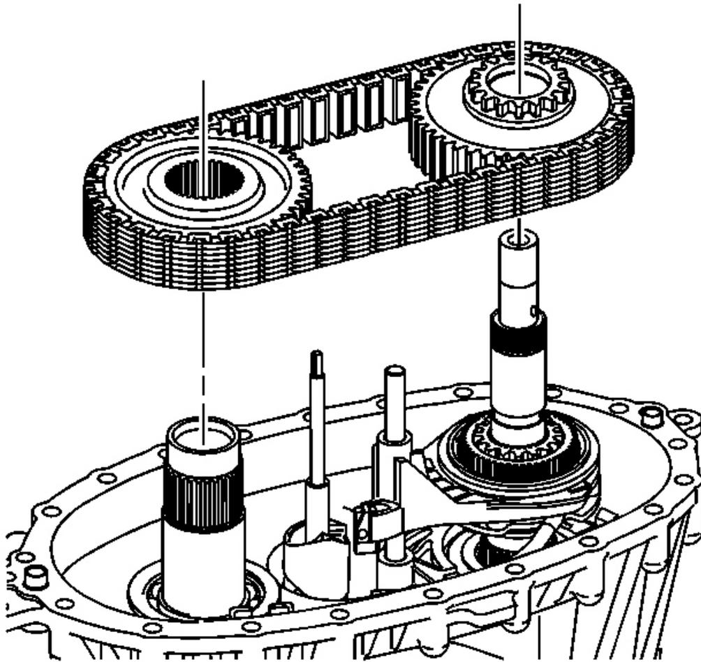
**Fig. 20: View Of Drive Chain & Sprockets**
