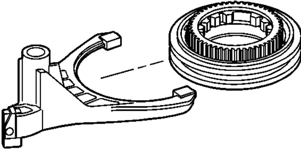
**Fig. 94: View Of Lockup Shift Assembly & Lockup Mode Shift Fork**
