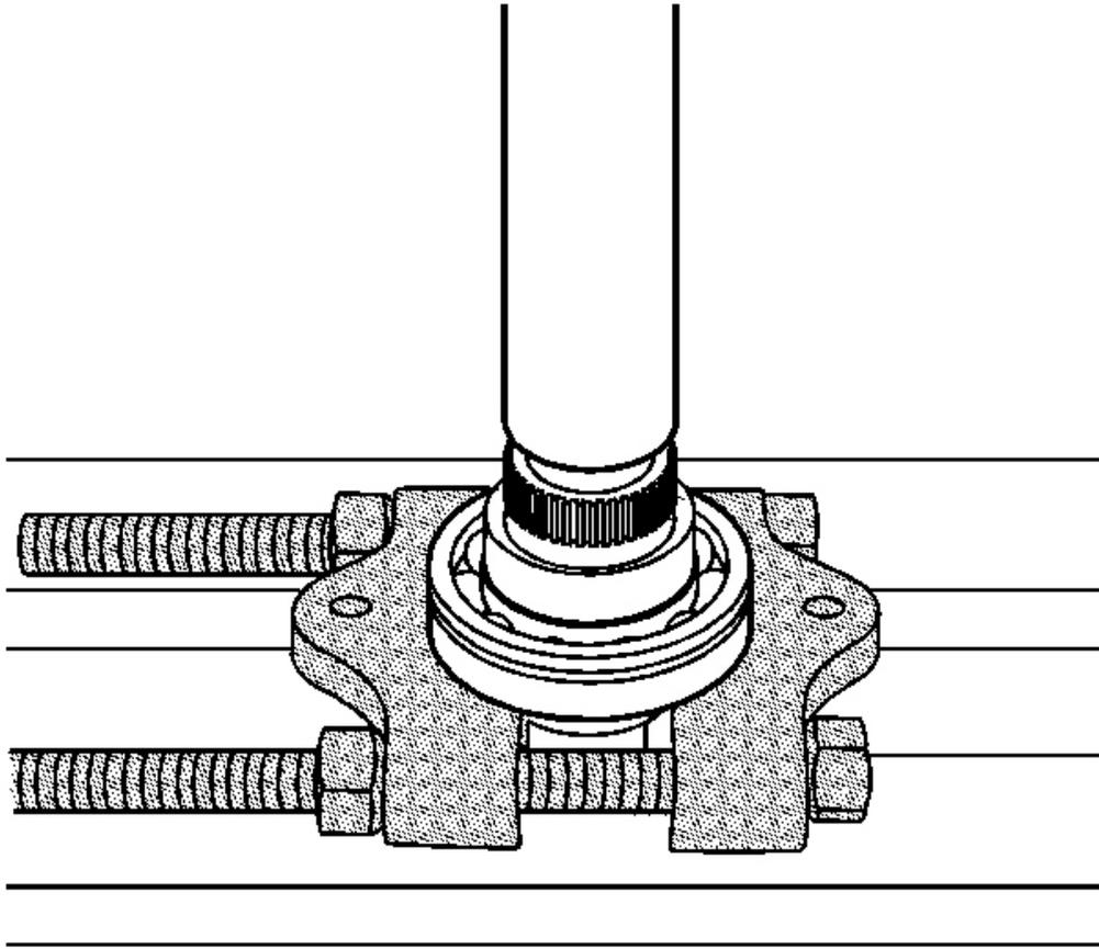
**Fig. 141: Installing Rear Output Shaft Bearing Using Hydraulic Press & J 22912-01**
