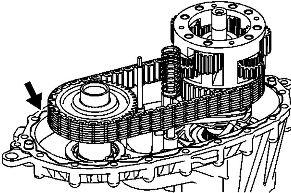
**Fig. 146: Applying RTV Sealant GM P/N 12345739 To Mating Surfaces Of Front Case Half**
