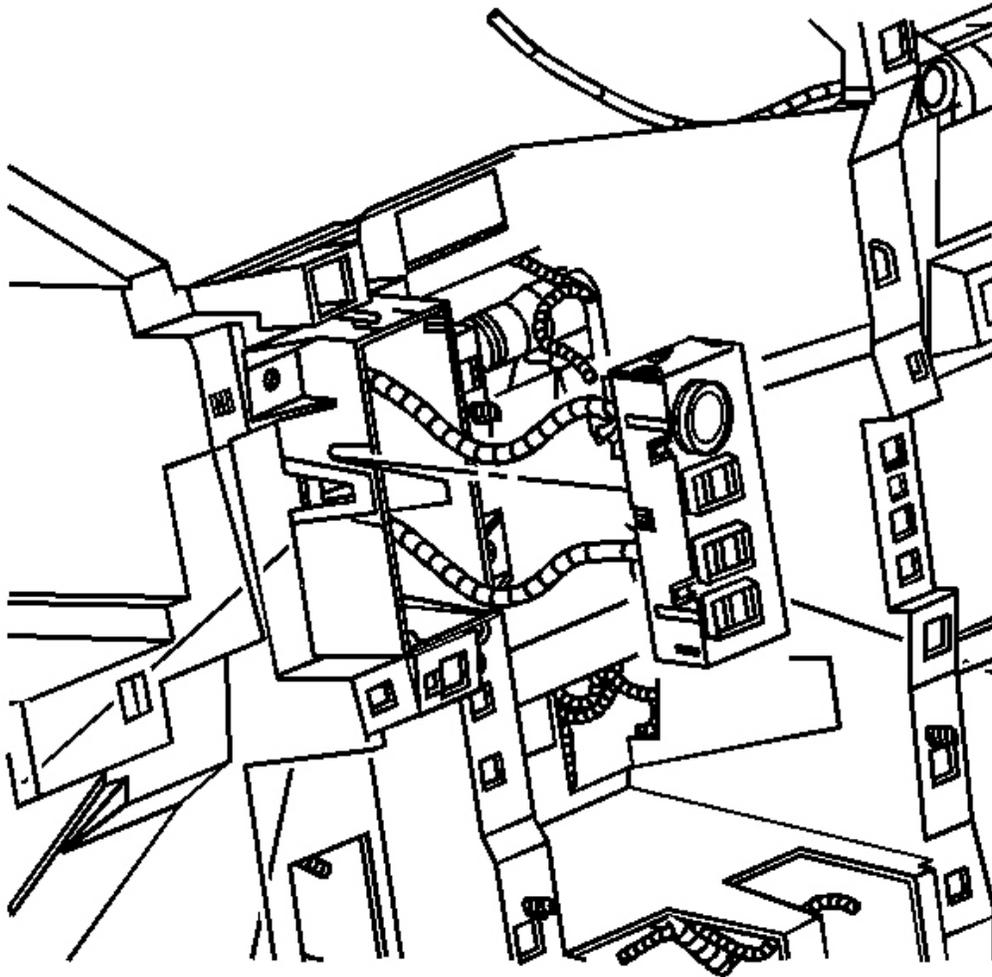
**Fig. 37: Shift Control/Selector Switch**
