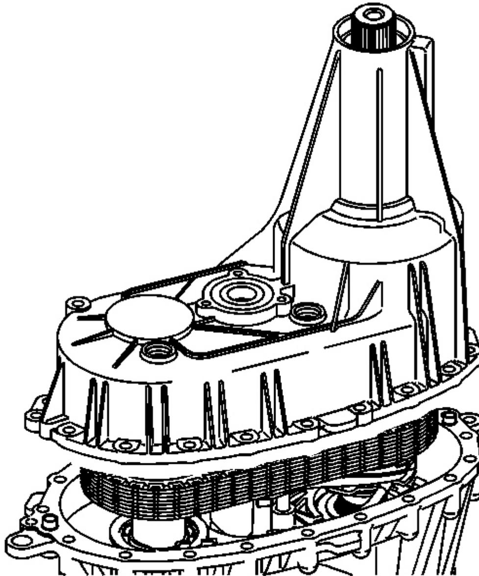
**Fig. 14: View Of Rear Case & Front Case Half**
