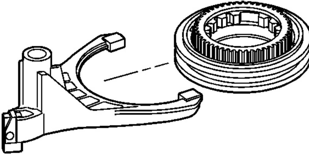
**Fig. 129: Lockup Mode Shift Fork & Lockup Shift Assembly**
