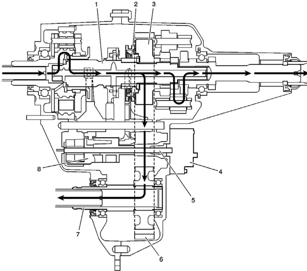
**Fig. 157: 4HI Lock Mode Power Flow**
