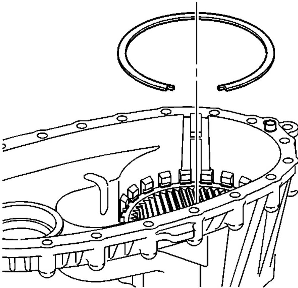
**Fig. 75: Locating Retaining Ring For Annulus Gear**
