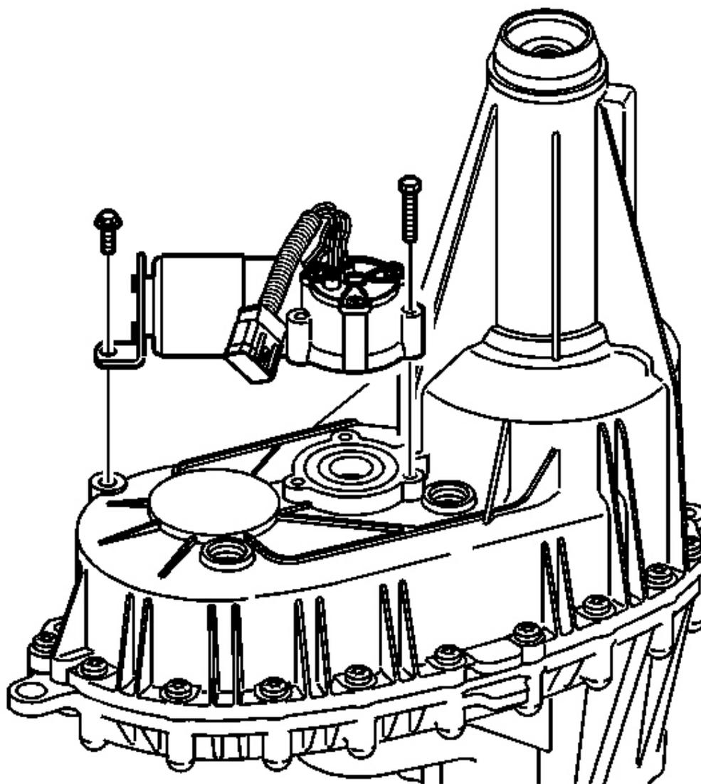
**Fig. 9: Locating Encoder Motor Assembly**
