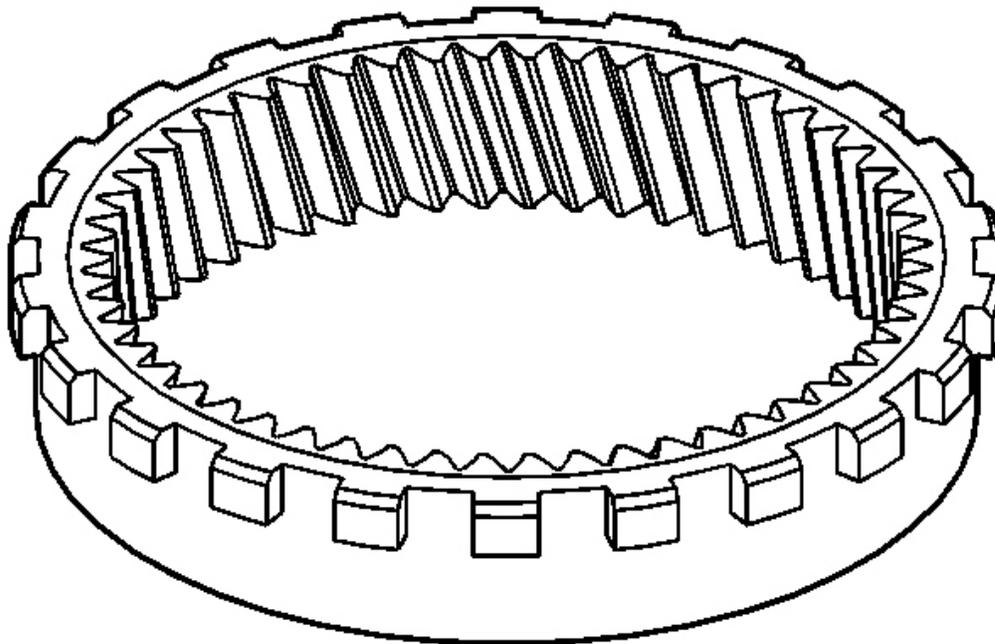
**Fig. 91: Inspecting Annulus Gear Teeth**
