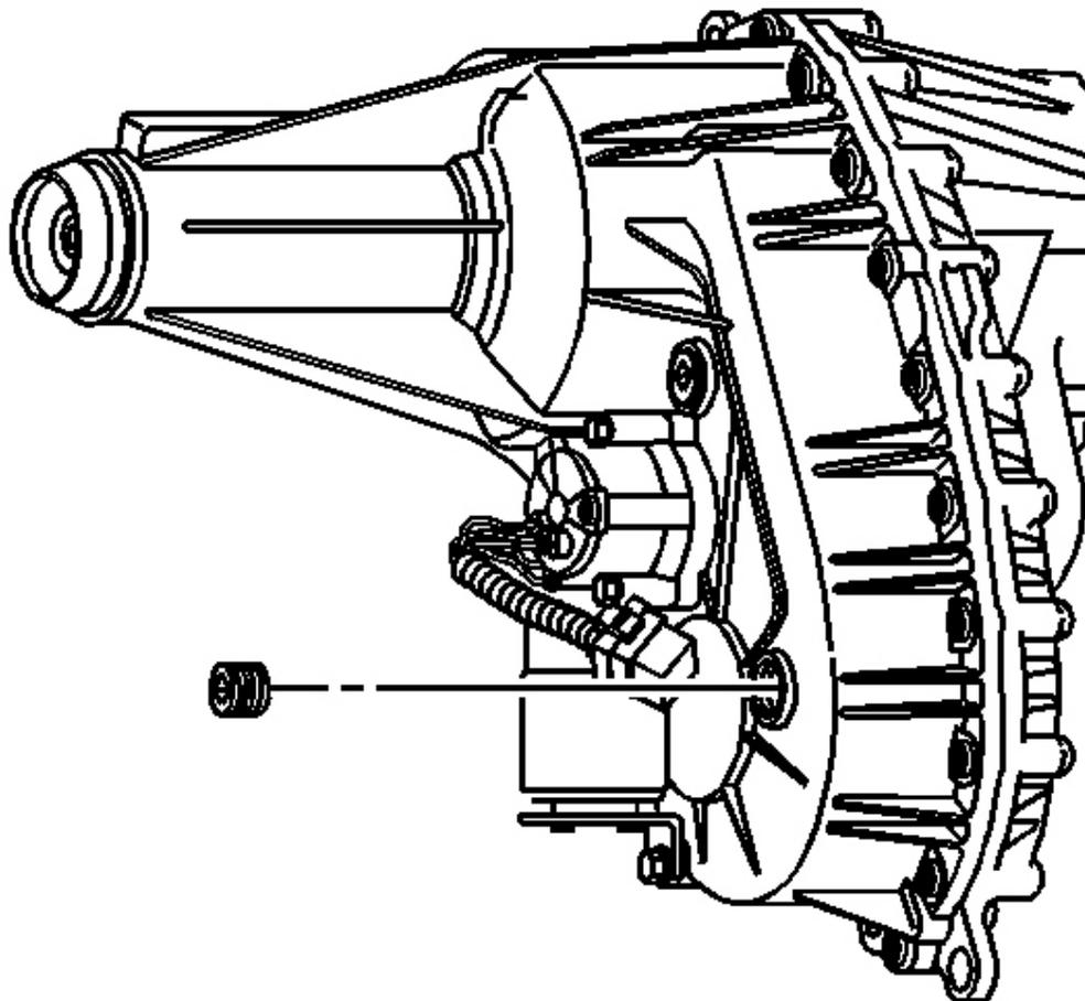
**Fig. 12: Transfer Case Drain Plug**
