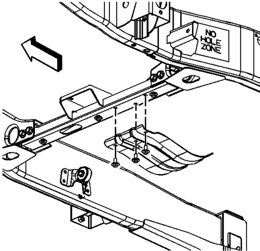
**Fig. 9: Transfer Case Shield**
